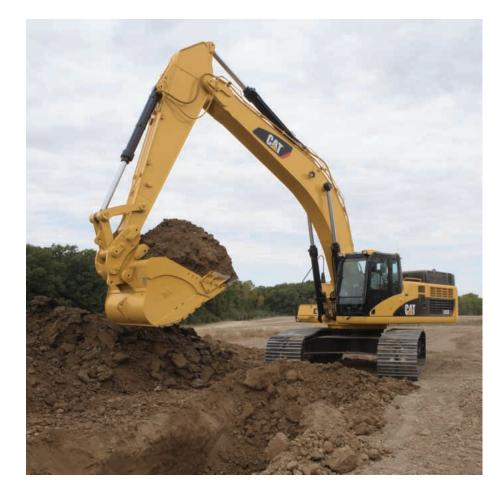
**Boom and Swing Priority.** The hydraulic system on the 345D provides automatic priority function for boom-up and swing operations eliminating the need for work mode buttons. When the boom or swing lever is activated, the system automatically assigns priority based on operator demand.
