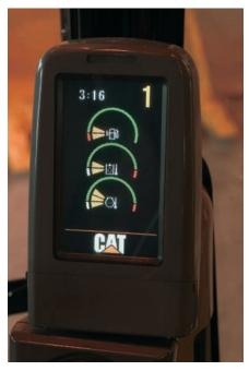
**Monitor Display Screen.** The compact, full color 400x234 pixels Liquid Crystal Display (LCD), displays machine maintenance, diagnostic and prognostic information, in twenty-seven different languages. The keypad allows the operator to select machine operation conditions and to set view preferences. The Master Caution Lamp blinks ON and OFF when one of these critical conditions occur:
