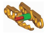
**Track.** The 345D comes standard with a grease lubricated track called GLT4. The track links are assembled and sealed with grease to decrease internal bushing wear, reduce travel noise and extend service life lowering operating costs. The track link for the 345D has been re-designed to avoid the concentration of stresses and improve durability and reliability.
