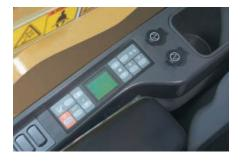
**Console.** The consoles feature a simple, functional design that reduces operator fatigue. Switch access is exceptional providing excellent visibility and easy operation. Both consoles have attached armrests with height adjustments.
