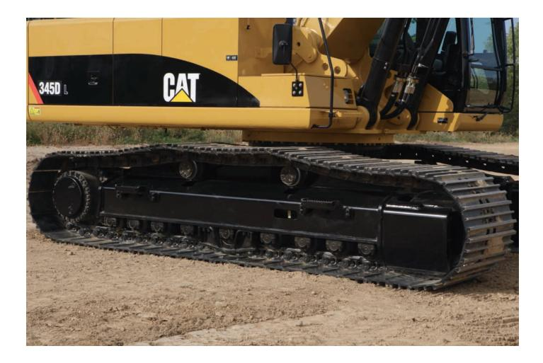
**Undercarriage Options.** Track with Positive Pin Retention 2 (PPR2) and cast idlers are available on the 345D. The PPR2 prevents loosening of the track pin from the track link and the cast idler is designed for extended life. Both options are ideal for extreme applications or those that require a large amount of travel.
