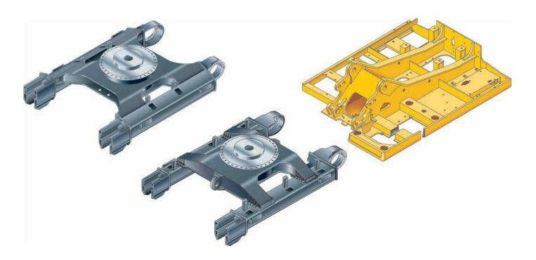
**Carbody.** The 345D has three undercarriage options to meet regional transportation requirements and application needs.
