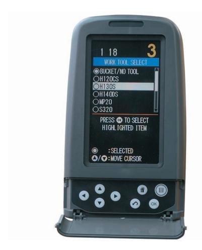
**Tool Control System.** The optional tool control system maximizes work tool productivity by configuring hydraulic flow, pressure, and operator controls to match a specific work tool. System versatility enables a wide range of tools to be used.
