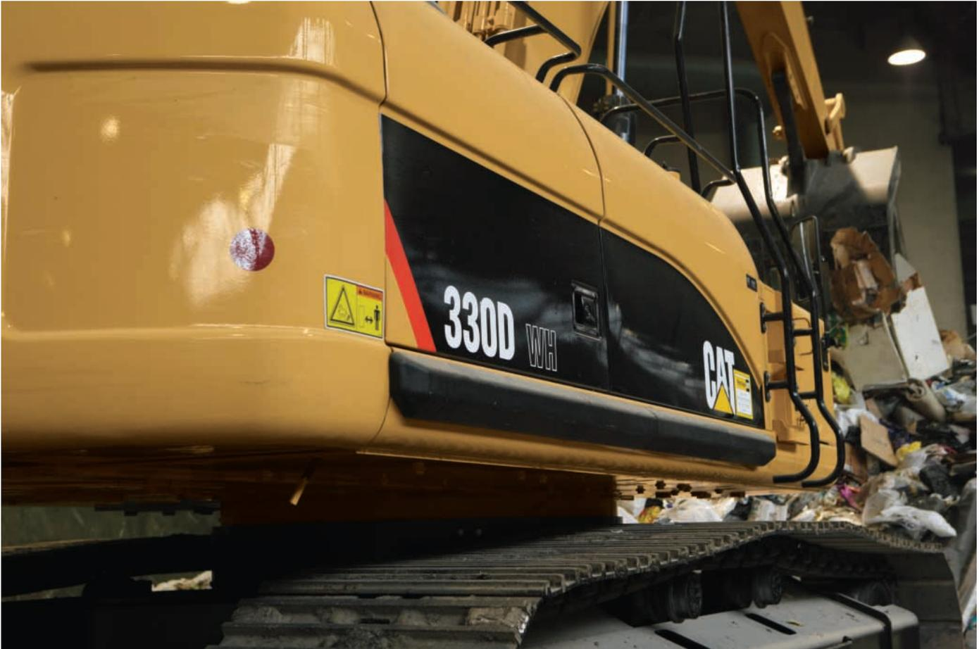
**Rubber Bumpers.** The rubber bumpers provide much needed guarding to protect the sheet metal of the machine from being damaged while maneuvering in tight areas.
