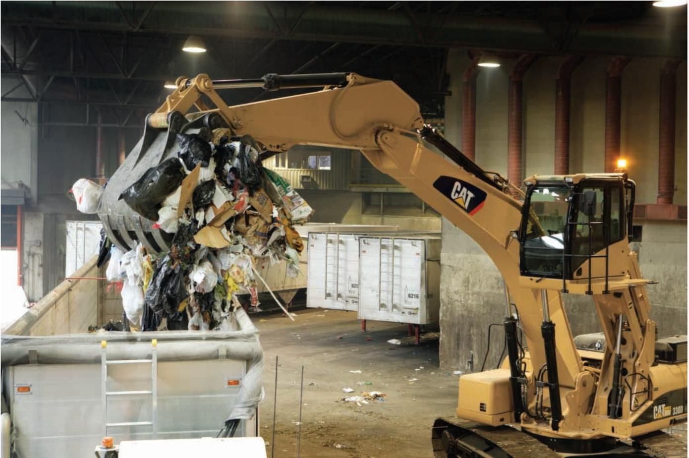
**Heavy-Duty Boom and Stick.** The heavy duty reach boom and heavy duty 3.2 m (10.5 ft) stick are more robust than the standard reach boom and stick. The “heavy-duty” features include thicker plates throughout the design to handle the increased loading experienced in transfer station applications.
