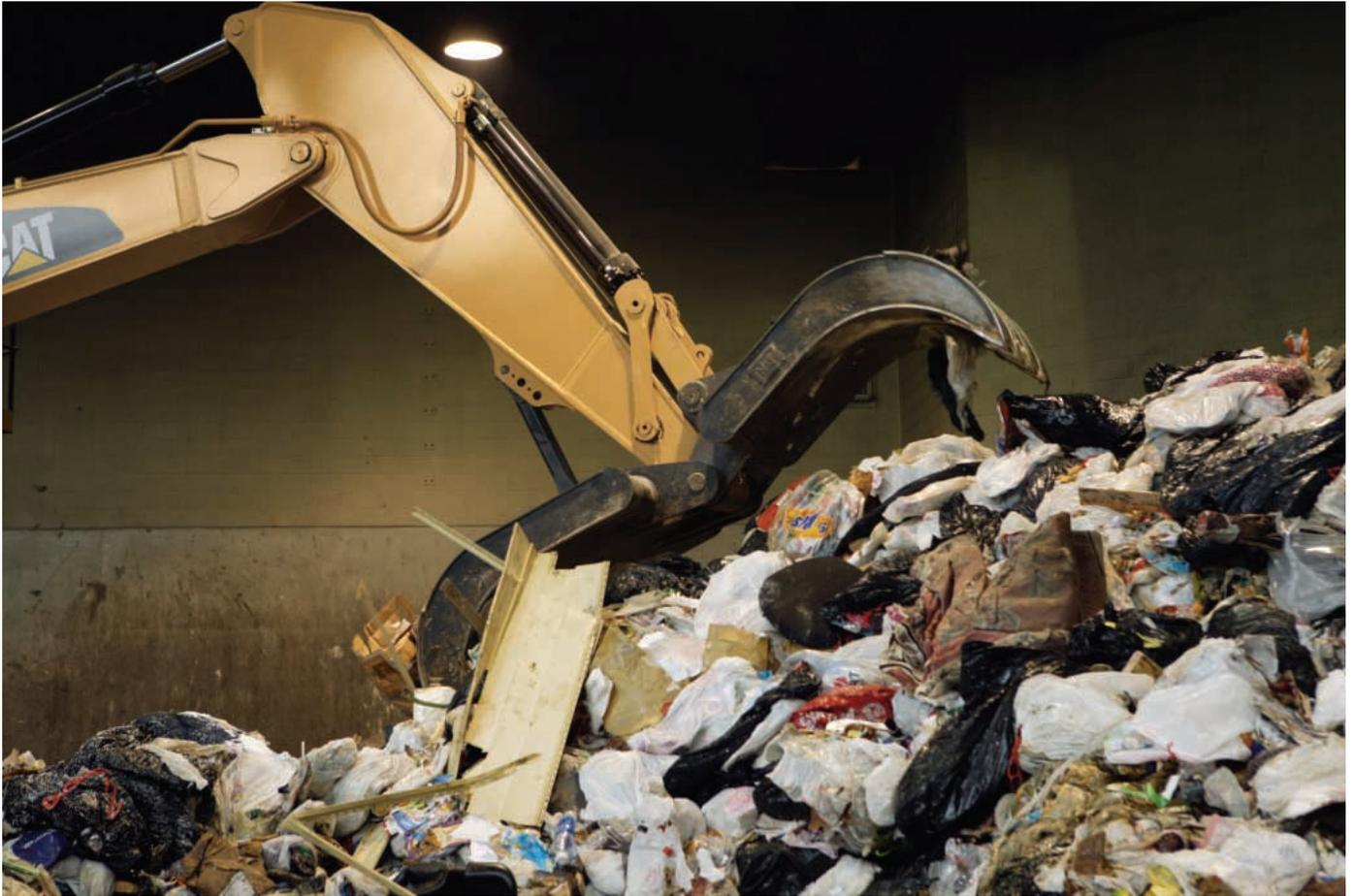
**Trash Grapple.** The Cat Work Tools trash grapple has been designed to meet the requirements of waste handling. Powered by the bucket cylinder, the trash grapple mechanically works to compact trash while placing it into the bed of the hauling unit. This helps to maximize the amount of waste that can be placed into one unit, maximizing efficiency.
