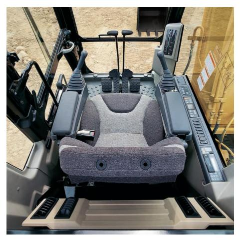
Redesigned Interior Layout. Redesigned cab layout emphasizes simplicity and ease of use. Right-hand wall and console provide easy access to all switches, dials and controls.
