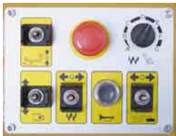
Left-side main screed control panel
