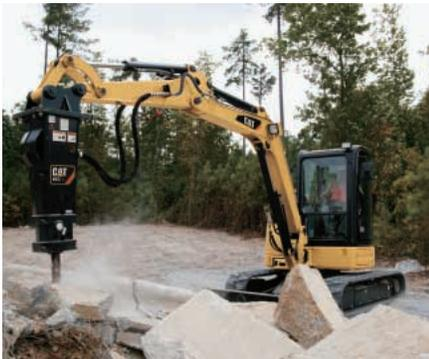
**Auxiliary Lines and Connectors.** The auxiliary lines and connectors including quick connections are fitted as standard, meaning the Cat 303C CR come ready to work. Hammer (one-way) and auger (two-way) auxiliary lines are also fitted as standard.
