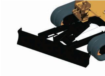
**Angle Blade Positioning.** The angle blade can be positioned straight ahead or angled up to 25 degrees to the left or right reducing the number of times required to back-up and reposition when backfilling thus reducing operation time.
