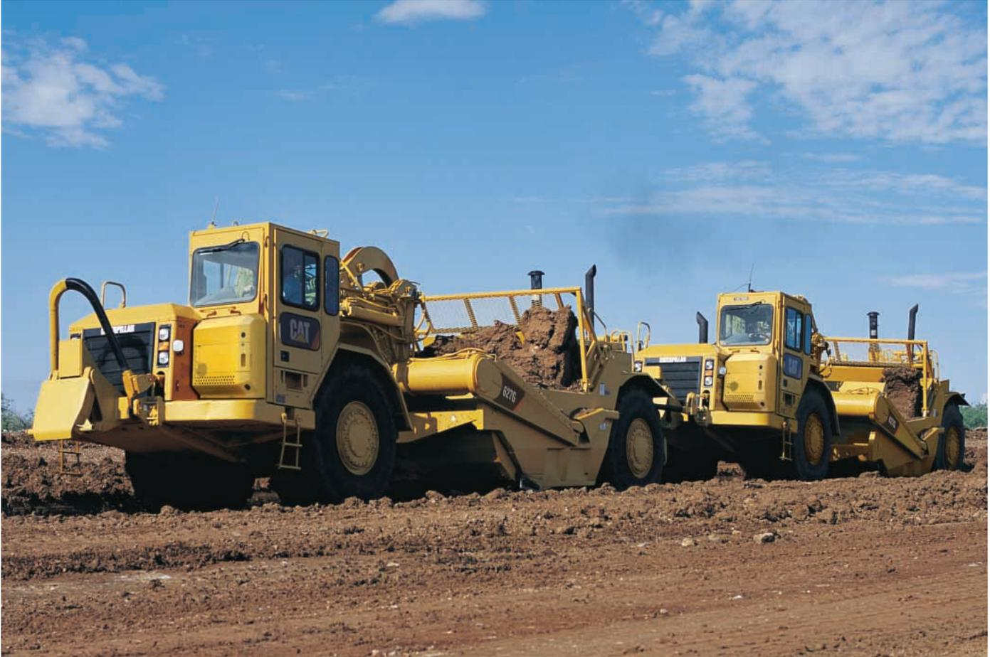
*Typical push-pull operation using twin 627G machines.*
