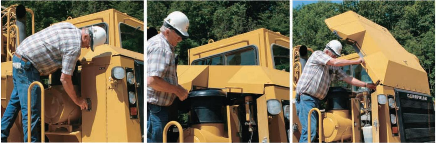
**Grouped Service Points.** Maintenance and service points for the engine are grouped on the right-hand side for easy access. They include the engine air cleaner, engine oil check and fill, fuel filters and priming, coolant level sight glass, window washer bottle, air conditioning dryer cartridge, ether starting aid canister, engine oil filter, fan drive lubrication, and sampling ports for the engine oil and coolant.
