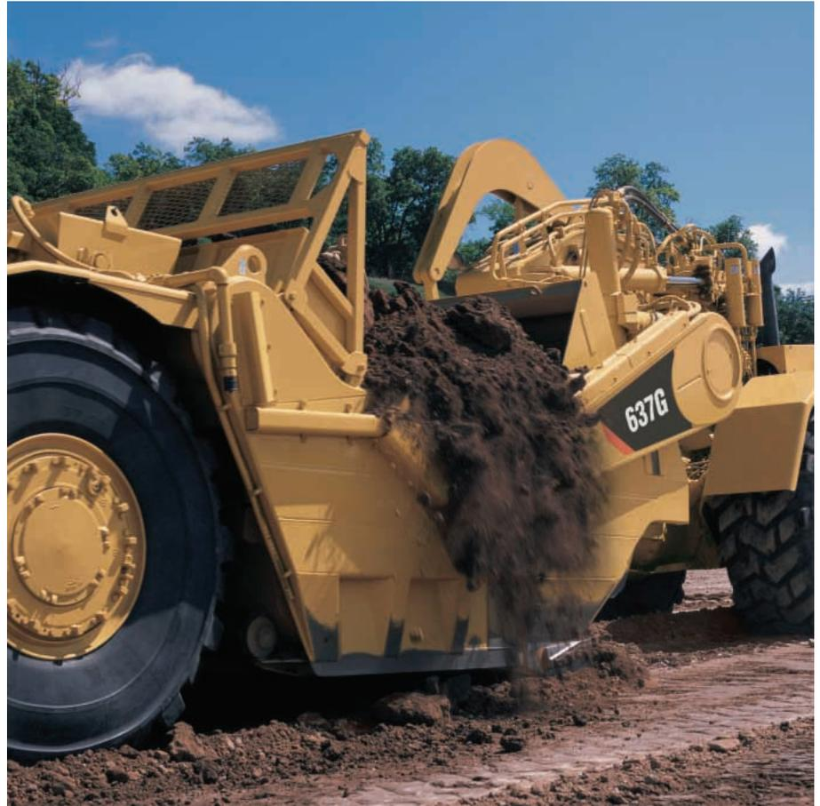
**Tandem Engine.** Two engines ensure the power to handle steep grades, and makes possible all wheel drive to handle soft, slippery underfoot conditions.
