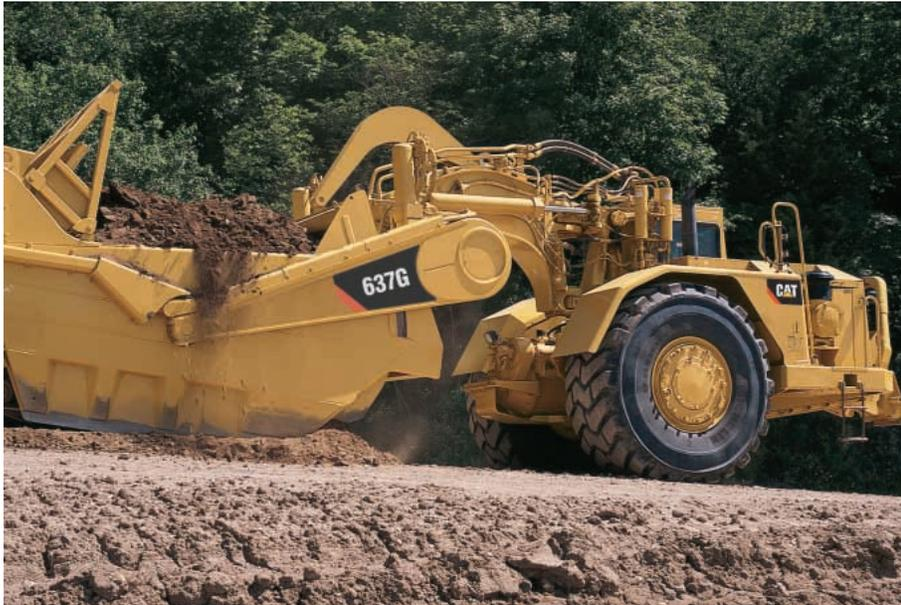
**Transmission.** Electronically controlled Caterpillar planetary powershift transmission with eight forward and one reverse speed. Tractor gears 1 and 2 operate in converter drive for increased torque capability during cut and fill operations. Gears 3-8 operate in direct-drive for drive train efficiency during the haul. All scraper gears operate in converter drive for increased torque capability during the cut and fill.
