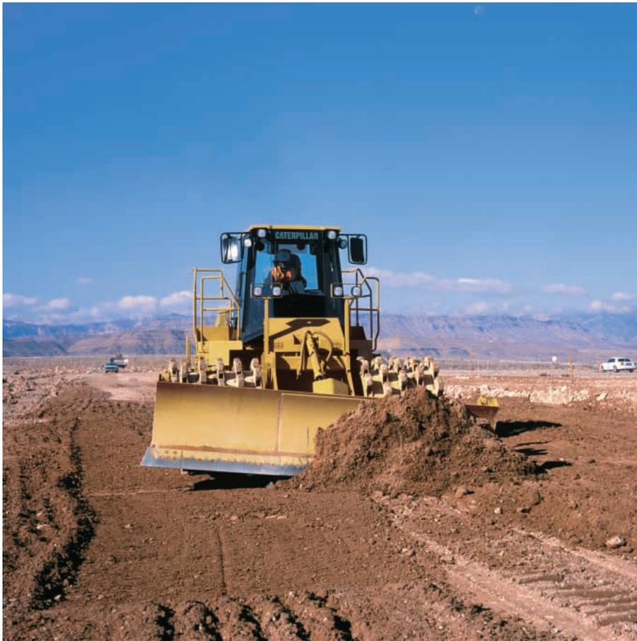
**Hydraulic System.** The hydraulic system provides low-effort blade control. Seat mounted levers send electrical signals to a pilot valve mounted on the front frame, moving the sound, heat and effort caused by the hydraulic valve out of the operator's station.
