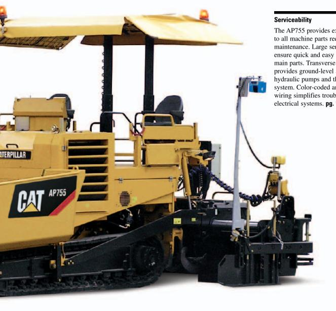
The AP755 provides excellent access to all machine parts requiring scheduled maintenance. Large service panels ensure quick and easy inspection of the main parts. Transverse engine mounting provides ground-level access to hydraulic pumps and the engine cooling system. Color-coded and numbered wiring simplifies troubleshooting of the electrical systems. pg. 10
