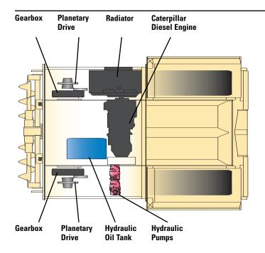
**Closed-loop hydrostatic propel system.** Provides accurate control of propulsion and low-maintenance operation.
