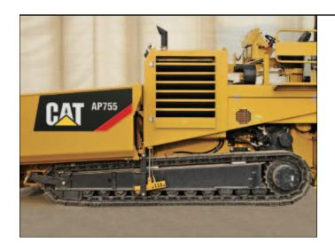
**Two rubber shoe crawlers.** The track-type asphalt paver provides a reliable, smooth ride. The optimum tension of the tracks is assured by a grease piston with a shock absorbing system.
