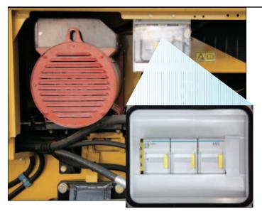
**Industrial, continuous-duty generator.** Working range from 1250 to 2200 rpm provides high reliability and low sound levels.
