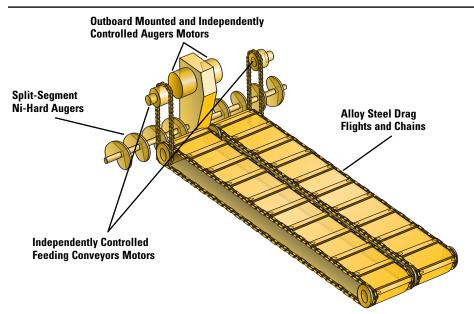
**Optimum productivity.** The material handling system allows the operator to maintain an uninterrupted flow of material from the hoppers to the screed. The system is responsible for maintaining the proper head of material - the volume of asphalt in front of and across the length of the screed.
