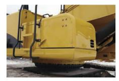
**Right Front Corner Genset.** The generator is now mounted on the right front corner of the machine upper to improve serviceability.
