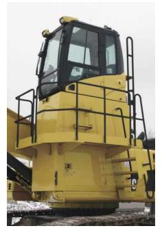
Caterpillar Designed and Built, 1.9 m (6'5") Cab Riser. The cab riser gets your operator to an operating height with excellent visibility for loading or unloading your processing equipment, trucks and rail cars. Access to the cab is provided by a platform which extends around the riser to allow windshield cleaning. The cab riser can also be manually tilted forward 90° for shipping.
