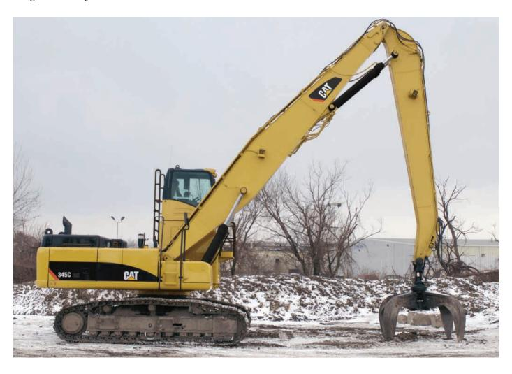
**Stick Options.** The 345C Material Handler is available with a choice of two different stick lengths. The 7.3 m (24'3") material handling stick which gives a 16.5 m (54'2") max-reach front linkage and the 9.1 m (29'10") material handling stick which gives a 18 m (59'0") max-reach front linkage.
