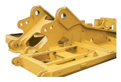
**Upper Frame.** Is specifically designed for the scrap and material handling market. It is built of higher strength material and thicker steel sections to handle the increased swing loads developed with the longer fronts and heavier counterweights used in material handling.
