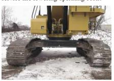
Wide 3720 mm (12'2") Track Gauge. Provides the over-the-side stability required to handle heavy loads and improve productivity. Carbody plates are 5 mm thicker than standard, high strength swing bearing bolts plus larger box-section height team up to provide superior joint retention and durability in material handling applications.
