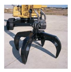
**Orange Peel Grapples.** The 1.5 yd<sup>3</sup> (1.15 m<sup>3</sup>) and the 2.0 yd<sup>3</sup> (1.53 m<sup>3</sup>) Orange Peel Grapples are available attachments.
