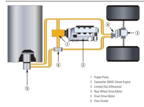
Single propel pump with flow divider provides separate, balanced hydraulic flow to the rear wheel axle and the drum drive motors. Provides high gradeability and increases tractive effort in loose or poor underfoot conditions. (Flow divider is optional on CS-323C without a leveling blade.)
