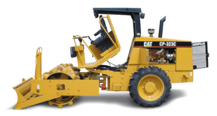
**Visual indicators** allow easy check of radiator coolant, hydraulic oil tank level and air restriction indicator.
