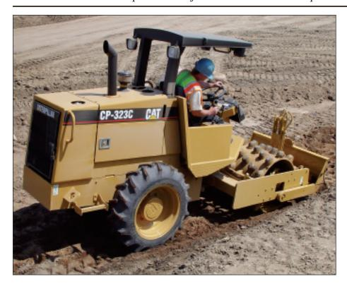
**Narrow machine width** of 1.39 m (4' 6") is ideal for working in trench applications or job sites with limited space.
