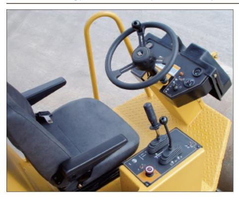
**Single lever control** for propel and vibratory On/Off provides simple and low effort operation.
