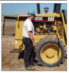
Daily service points are accessible from ground level and are grouped on one side of the engine. The optional hinged side access doors open wide for easy access to engine components.
