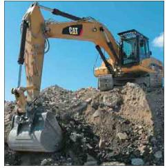
**Tracks.** The 325D comes standard with grease lubricated tracks. The track links are assembled and sealed with grease to decrease internal bushing wear, reduce travel noise and extend service life lowering operating costs.
