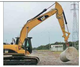
**Heavy Lift Mode.** Maximizing lifting performance and boosting the lifting capability. Heavy loads can be easily moved in the full working range of the machine maintaining excellent stability.
