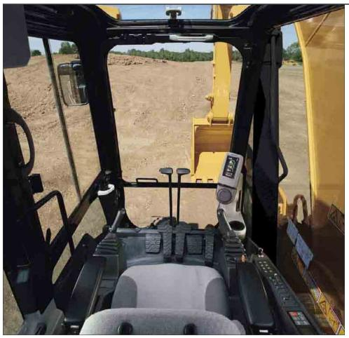
**Operator Station.** The workstation is spacious, quiet and comfortable, assuring high productivity during a long workday. The air conditioner and attachment switches are conveniently located on the right-hand wall, and the key switch and throttle dial are on the right-hand console. The monitor is easy to see and maximizes visibility.
