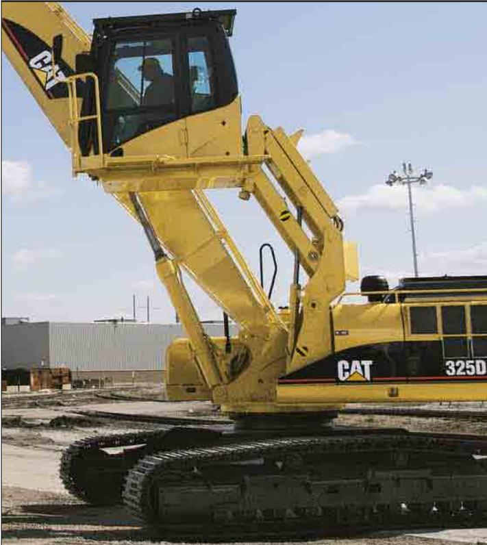
**Hydraulic Cab Riser.** The new design of the parallelogram hydraulic cab riser offers increased visibility as well as optimized operator comfort thanks to higher, larger and more robust structures. The activation of the hydraulic cab riser is modular, and thus, allows the operator to control the riser speed and decrease shocks. In case of emergency, the cab can be lowered while using a safety lever either inside the cab or inside the radiator compartment.
