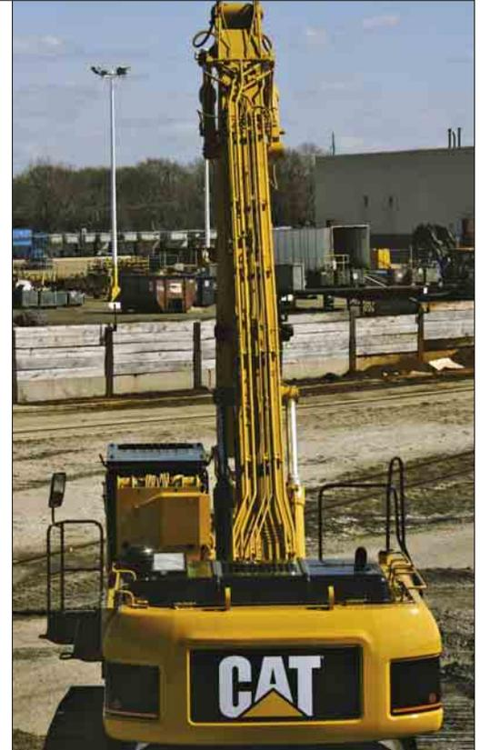
**Heavy Lift Mode.** The operator can select the heavy lift mode at the push of a button to boost lifting capability and provide improved controllability of heavy loads.
