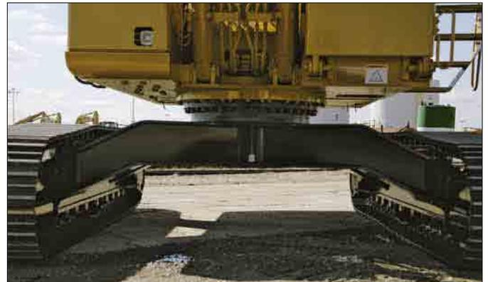
**Square Undercarriage.** An optional long, heavy duty, high and square undercarriage maximizes the over-the-side stability and improve productivity. Lifting capacities are improved over-the-side required to handle heavy loads.
