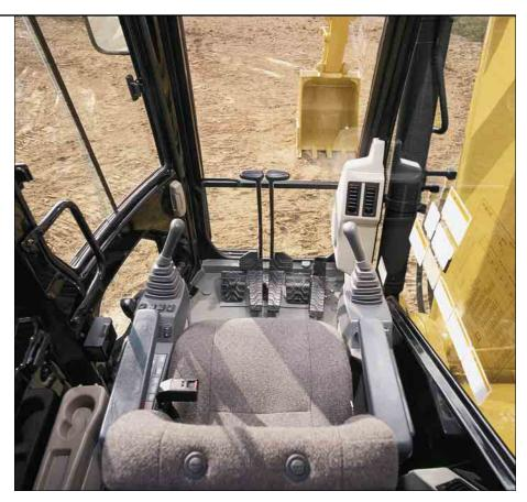
**Travel Controls.** The footrest provides a more comfortable way to control the travel pedals. The two travel control levers have a reverse-L shape, making them easier to operate. Lever stroke and force have been adjusted to improve fine control and to prevent jolting during travel.
