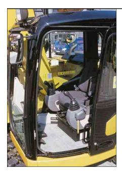
**Sliding Door.** The cab door slides alongside the cab and takes less space to open and close than a hinged door. This unique design allows the operator to easily get in and out of the cab when working against walls on job sites, even when attachments are added.
