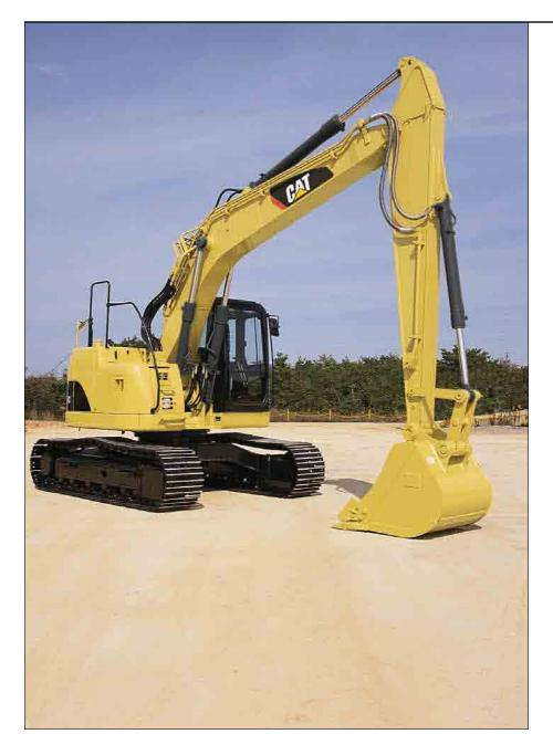
**Front Linkage Attachments.** Allows the use of one boom, two sticks and five buckets. Using these combinations makes the excavator productive in a wide range of applications.
