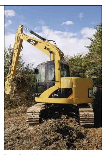
**Compact Radius Design.** The 314C LCR features a compact radius, making it ideal for working in tight areas.
