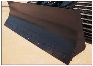
**Blades.** Three blade widths are available as attachments. The bolt-on cutting edge consists of three pieces, which can be reused by turning them upside down. Replaceable bolt-on edges protect the blade from damage and wear. Mesh bearings in the pin joints of the blade cylinder extend the greasing interval.
