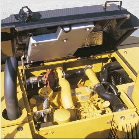
**Cooling System.** A large-diameter fan and full-length, water-cooled cylinders, combined with excellent thermal efficiency, help prevent overheating. The result is longer engine life and the ability to operate at high temperatures and under heavy loads. The core radiator is equipped with waved fins to prevent clogging.
