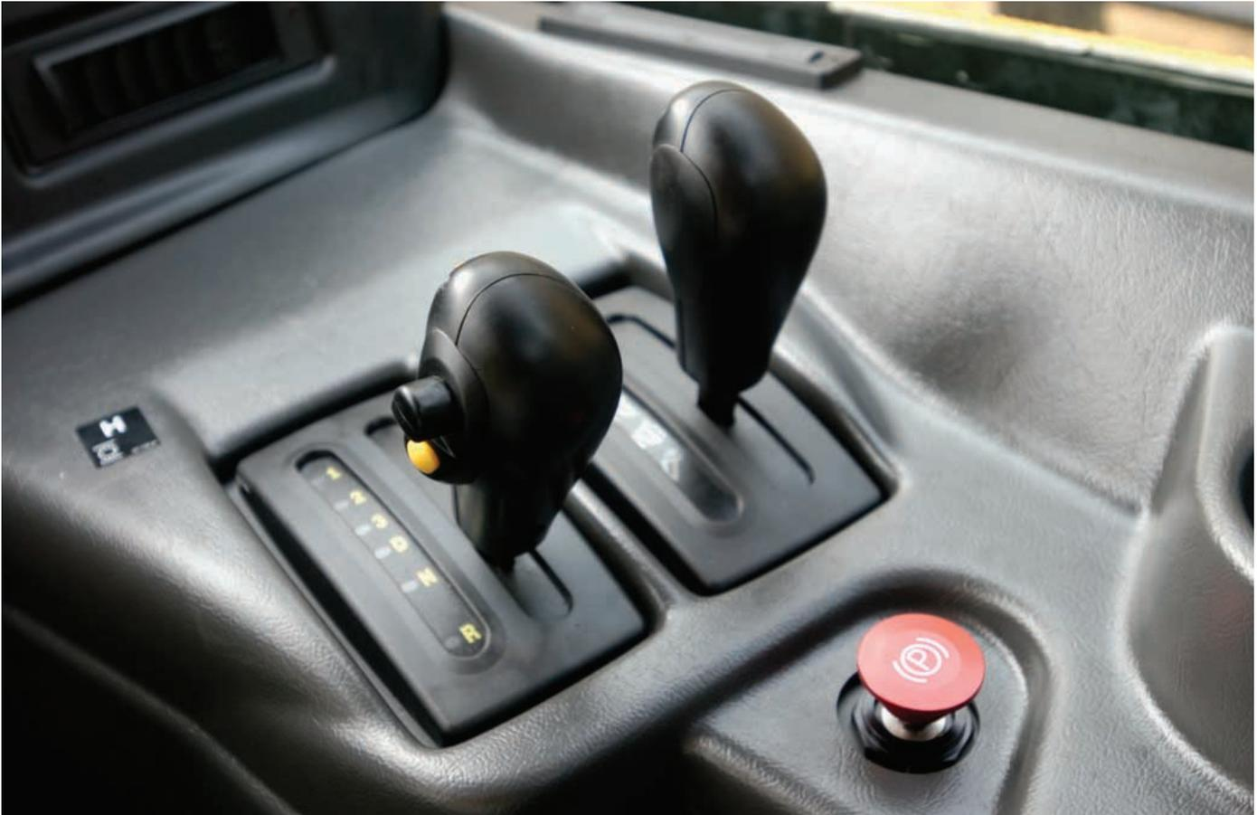
**Ergonomic Layout.** The controls and layout of the cab are designed to make it as easy to operate as your car. Quick and easy to read and simple to operate, the controls on the 725 allow the operator to concentrate on production.
