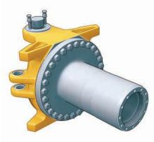
Hitch Construction. Two-piece bolted hitch features a strong, durable cast steel head bolted to a hard wearing forged steel tube. The hitch tube has large hardened bearing areas and a hardened thrust face for reduced maintenance and longer life.
