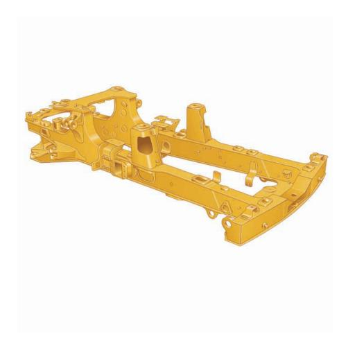
**Front Frame.** The front frame design features a large box section and wide, stiff frame beams to handle torque loads. The divergent frame design decreases stress in the hitch area and optimizes suspension geometry. The frame design makes maximum use of robotic welding for increased durability.
