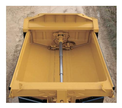
**Carry-Back.** The design of the ejector is inherently self-cleaning and practically eliminates material sticking to the body, which increases productivity, improves fuel efficiency and lowers cost per ton.
