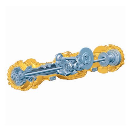
**Front Suspension.** The three-point front suspension permits the axle to oscillate  $\pm 6^{\circ}$ , softening impact loads on structures and components and providing a smooth ride, so the operator can travel at speed over rough terrain.
