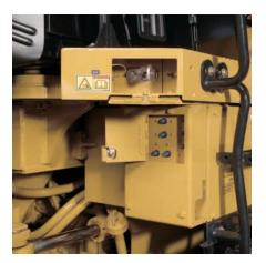
relay panel and an optional tool box are conveniently located below the left-side access platform. The engine shutdown switch is housed with the relay panel. A compartment integrated into the access platform contains the hood tilt actuation switch, master switch and jump-start receptacle.
