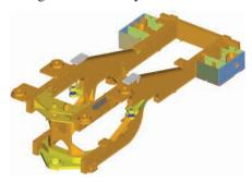
**Engine End Frame (EEF).** A full box-section engine end frame with hitch plates at the front end provides a strong, rigid structure that resists twisting and impact loads. The result is an extremely solid mounting platform for the engine, transmission, axle, ROPS and other accessories.
