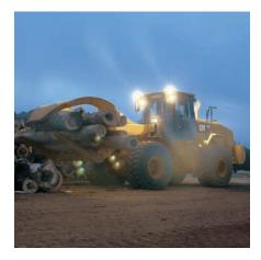
Lighting Packages. Optional lighting packages are available for roading or low-light applications. The optional High Intensity Discharge (HID) lights provide exceptional lighting for night work. A rotating beacon is available as a safety feature.
