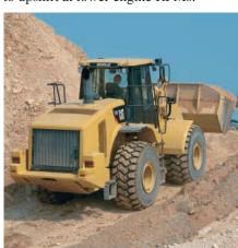
**RIDE CONTROL.** The optional Ride Control System improves ride, performance and load retention when traveling over rough terrain. Operators gain confidence moving at higher speeds in load and carry operations decreasing cycle times and increasing productivity.
