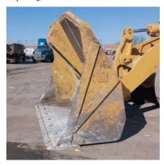
**Waste Buckets.** Waste buckets are designed for long life in the harsh world of refuse applications. This high-capacity bucket is well-suited for loading, sorting and other transfer station work.
