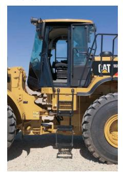
**ENTRY AND EXIT.** A ladder with self-cleaning steps keeps debris build-up to a minimum. The ladder is at a 5° forward incline for easy entry and exit.
