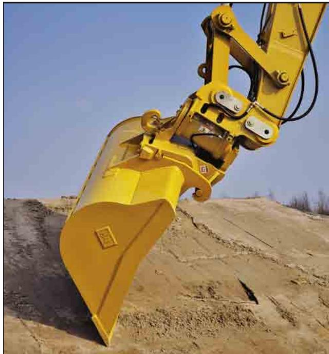
**Rationalized Bucket Line.** Optimized design matches machine configuration perfectly. Improved balance between performance and durability. Buckets feature the Caterpillar K Series Tooth System.
