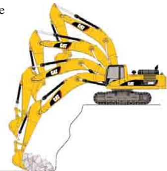
**Truck Loading.** Loading trucks from a bench is more productive and fuel efficient as the return cycle is reduced while the boom down function does not require pump flow.
