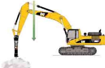
**Hammer Work.** The front parts automatically follow the hammer while penetrating the rock. Blank shots or excessive force on the hammer are avoided resulting in longer life for the hammer and the machine. Similar advantages with vibratory plates.
