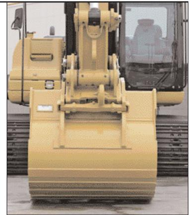
**Bucket Linkage.** Two bucket linkages (DB and TB) are available, with lifting eye on the power link.
