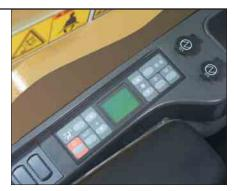
**Consoles.** Redesigned consoles feature a simple, functional design to reduce operator fatigue, ease of switch operation and excellent visibility. Both consoles have attached armrests and allow the height of the armrests to be adjusted.
