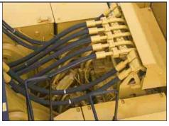
Component Layout. The hydraulic pumps, control valve and hydraulic tank are located close together to minimize the length of piping. The swing control valve is mounted directly on the swing motor. Main and swing pump suction and discharge lines have large diameters. These large diameters, combined with the component layout, guarantee high efficiency.
