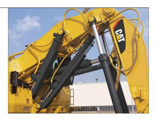
Linkage Pin. All pins used in the 385C FS front linkage have thick chrome plating, giving them high wear and corrosion resistance. The diameter of each pin is made as large as possible to smoothly distribute the shear and bending loads associated with the digging and lifting forces.
