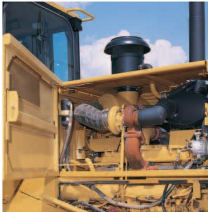
**Left Side Service Access.** Provides convenient entry to the engine oil filter, grease points, air filter, power train oil dipstick, coolant sight gauge, power train oil fill, power train oil filter and high speed engine oil fill.
