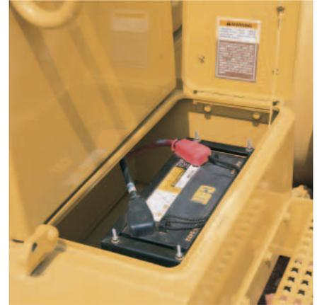
**Battery Box.** Is located in the right side bumper for convenient access to the maintenance-free batteries.
