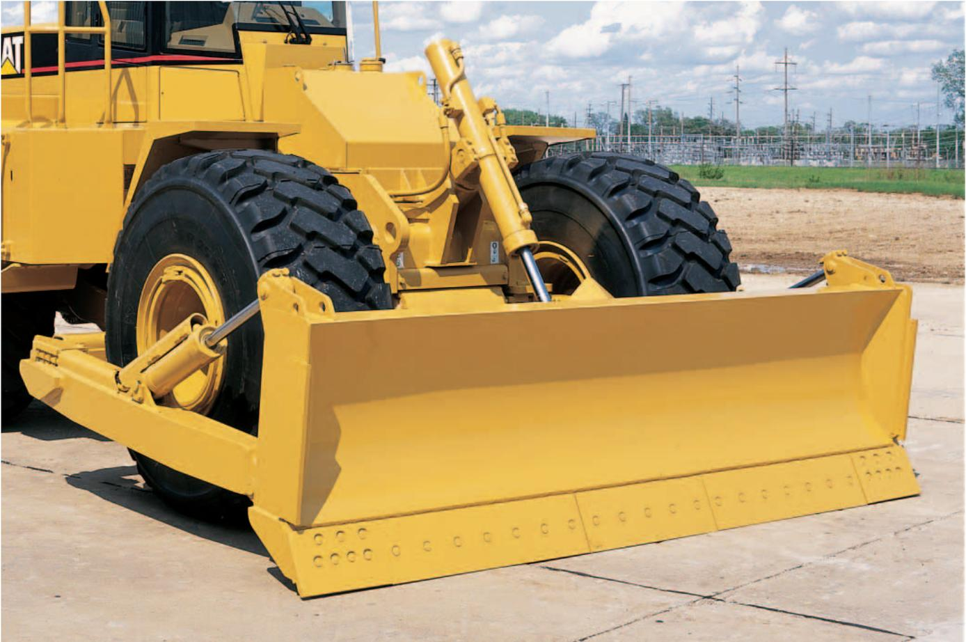
**Blade Package.** Consists of blade, push arms, trunnion mounting, dozer length skid plate, reversible cutting edges, self-sharpening end bits, hydraulic lines guard and hydraulic blade cylinders.
