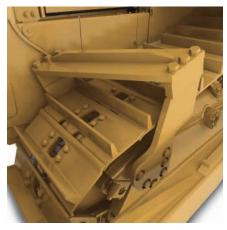
**Front Striker Bars.** The front striker bars angled design prevents debris from riding up the track and damaging the fenders or fuel and hydraulic tanks.
