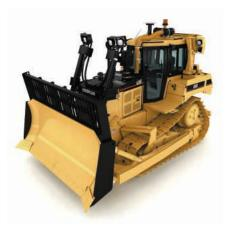
Black Painted Hood, Cylinders, and Back of Blade. The black painted hood, cylinders, and back of blade reduces glare from lights while operating at night and while operating in direct sunlight.
