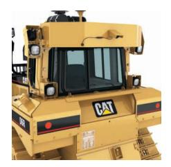
Rear, Tank-mounted Lights. The rear, tank-mounted lights are relocated on the ROPS, which removes the lights from the concentrated debris environment to help protect them from damage. Combinations vary depending on each model.
