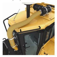
**Enhanced Cab.** The enhanced cab provides higher cab pressurization for improved cab air quality in dust and debris-laden applications. Includes a powered precleaner, with a high efficiency filter, which reduces system maintenance intervals.
