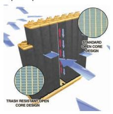
Radiator (AMOCS) (D7R II). The AMOCS radiator utilizes an exclusive two pass cooling system and increased cooling surface area to provide significantly more cooling capacity than conventional systems. A trash core radiator is available with six fins per inch, replacing the standard nine fins per inch.
