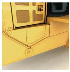
**Chassis Guards.** The chassis guards help protect the engine compartment by deflecting debris from rising upward along the chassis.
