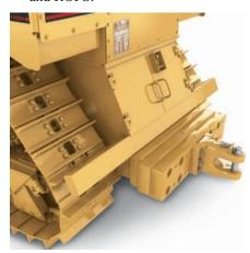
**Rear Striker Bars.** The rear striker bars incorporate a rigid drawbar and housing with large access doors for storage on machines not equipped with rippers. The rear striker bars are counterweight-ready in case additional rear weight is needed. For machines with rippers, striker bars mount on ripper frame.
