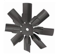
**Ejector Fan.** The ejector fan blade is designed with curved edges to help throw debris out radially. This helps prevent debris from clogging the radiator.
