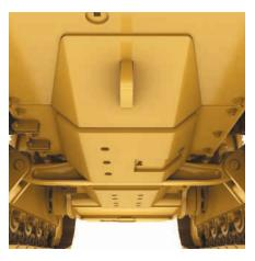
**Extreme Service Crankcase (bottom) Guards.** The crankcase (bottom) guards serve a dual purpose. They help prevent contact damage to vital power train components, and help keep debris out of the power train compartments.
