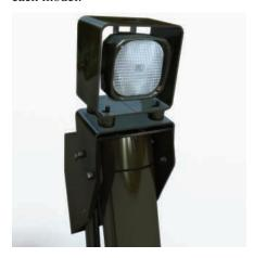
**Front Lights.** The front lights are mounted on top of the bulldozer lift cylinders allowing them to project light over the trash rack and keep the lights above the concentrated debris environment for longer service life.
