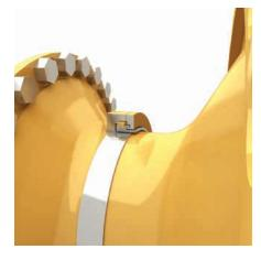
Final Drive Seal Guards. The final drive seal guards help prevent wire, nylon strapping, etc., from wrapping around and damaging the Duo-Cone seals. The outer guard is now stationary, thicker, and has increased hardness, all of which help prevent excessive wear from debris.
