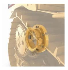
**Clamshell Guards.** The clamshell guard provides a non-rotating guard installed over the final drives to help prevent wire wrap. The guard includes inspection plates.
