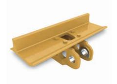
**Trapezoidal Hole Track Shoes (D7R Series II).** The trapezoidal hole track shoes reduce refuse packing within the track and reduces track chain tightening and accelerated pin and bushing wear. The trapezoidal holes relieve packing by allowing the sprocket to punch out dirt and debris.
