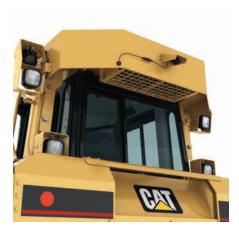
ROPS-mounted Air Conditioner Condenser and Fans. The ROPSmounted air conditioner condenser and fans are mounted to the back of the ROPS to maintain overall machine height.
