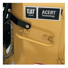
**Heavy-duty Handles.** The heavy-duty handles are manufactured from solid rod to withstand the rigors of landfill operation.
