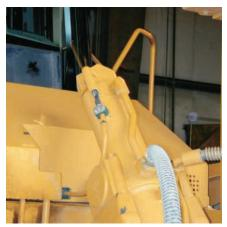
Automatic Blade Positioning. Operator automation is provided through the use of in-cylinder sensors and implement software.
