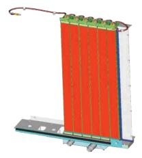
**Next Generation Modular Radiator** (**NGMR**). The parallel flow system with six cores standard (seven on the high ambient machine) improves cooling capabilities. Serviceability is also enhanced as there is no top tank to remove. The NGMR uses copper brazed brass tubes and copper fins.
