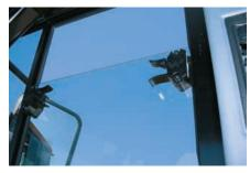
**Optional Sliding Cab Window.** Located in the right and left doors are optional sliding windows to provide access to outside air without opening the door.
