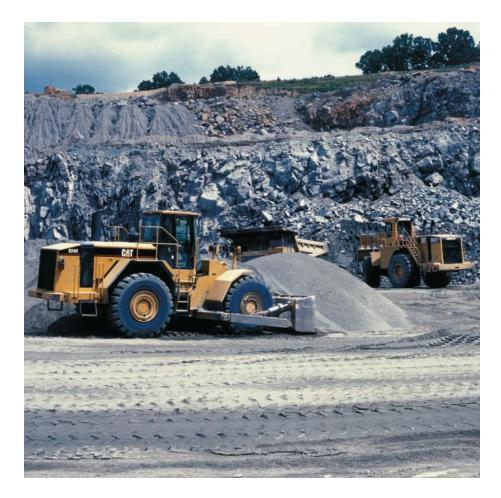
**Secondary Brake.** The secondary brake can be applied manually by the operator. In addition, the Caterpillar Monitoring System alerts the operator if pressure drops and will automatically apply the parking brake. **Cold Start.** This feature is improved by not only ADEM IV but also a new larger starter and four higher CCA batteries (1000 CCA).
