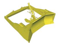
• Extended Wear Bulldozer Arrangement. The Extended Wear bulldozer arrangement is designed for moving large loads over long distances in harsh conditions. It consists of a 6.9 m<sup>3</sup> (9 yd<sup>3</sup>) U-blade with Abrasion Resistant Material (ARM) on the front and sides, cutting edges, push arms and integrated cylinder guards, and a heavy-duty stabilizer.
