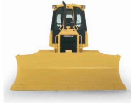
**VPAT Blade.** The VPAT blade is specifically designed for finish grading, backfilling ditches, cutting V ditches, windrowing, fill spreading, medium land clearing and heavy dozing. VPAT blades are built with four full-width (three on intermediate and LGP), box-section reinforcement cells for unmatched strength and durability.
