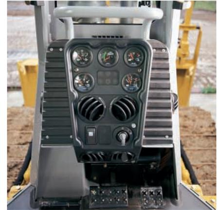
**Monitoring Package.** The monitoring package allows the operator to be aware of system conditions without having to constantly view gauges. Fuel level, hydraulic oil temperature, oil pressure, coolant temperature, and maximum speed setting gauges are all included in the instrument panel. Indicator lamps warn operator of:
