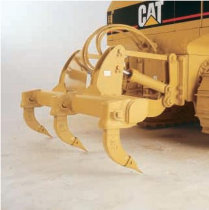
**Parallelogram Ripper.** This new, larger tool is more aggressive and allows the operator to do more effective ripper work. Heavy duty design provides long life. Parallel linkage design allows for better penetration and maneuverability in tight working areas. A longer shank delivers more work per pass making the machine more productive.
