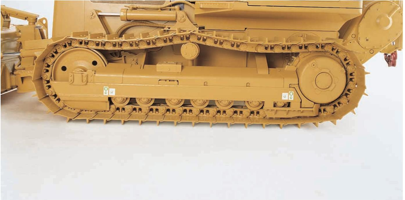
**Durable Components.** Advanced metallurgy processes produce improved life for bushing and sprocket segments. Segmented sprockets (standard equipment) offer easy serviceability and low replacement cost compared to replacing the complete sprocket hub. Caterpillar undercarriages are designed for long wear and lower owning and operating costs.
