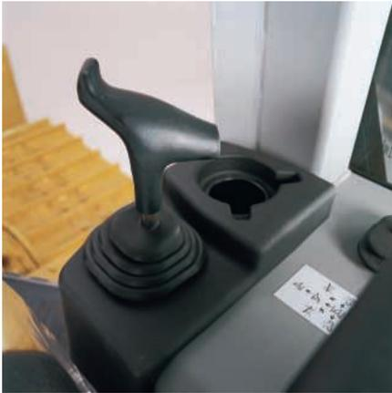
**VPAT Dozer Control.** A single lever control handle is used to control all blade lift, angle and tilt functions. The ergonomically designed handle fits comfortably in the operator's hand and delivers superb grading results.
