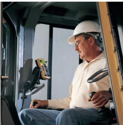
**Advantages.** Current earth moving and fine grading processes are labor intensive, dependent on manpower and instruments. Maintaining consistent grade between grade stakes is challenging, even for experienced operators. The AccuGrade Laser Grade Control System reduces labor requirements, aids operators in maintaining a consistent grade across the worksite and reduces material cost.
