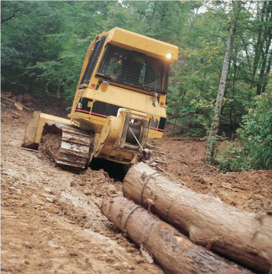
**Hydrostatic Winch.** Previous mechanical winches were driven by shafts and controlled by brakes and clutches. This new winch is driven by its own closed-loop hydrostatic system consisting of a variable displacement hydraulic piston pump and motor.
