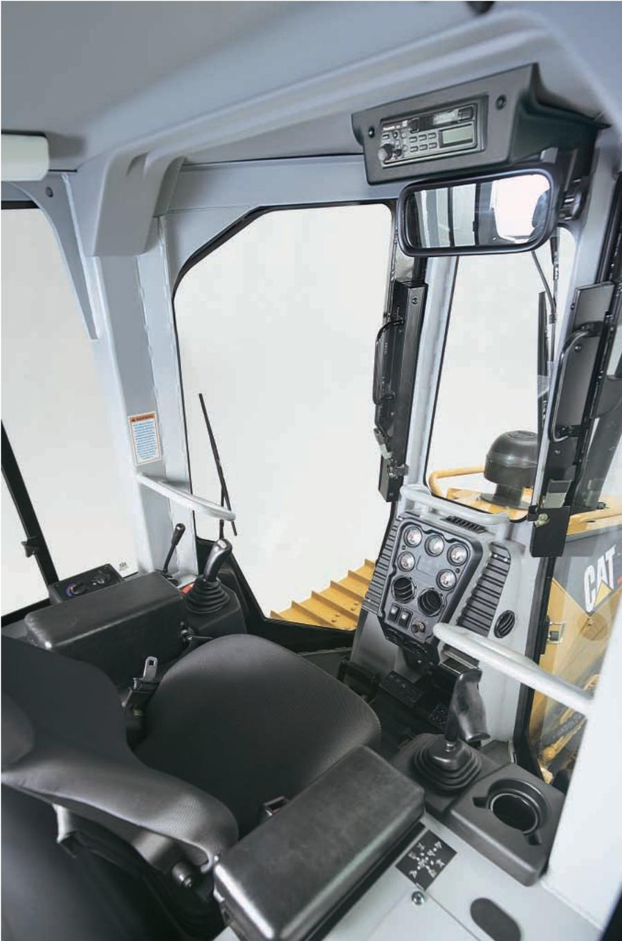
**Redesigned Operator Station.** Based on the cab designs of the large Caterpillar track-type tractors, the operator station has been redesigned to be more spacious. The new ergonomic layout emphasizes simplicity, ease of use and comfort. A new climate control system (HVAC), increased leg room and enhanced visibility allow the operator to focus on the job. With 13% more tinted glass area, the operator station provides a clear view to the blade and the surrounding work site.
