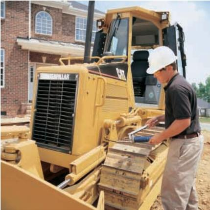
**Improved Pin Joints.** Pin joints have been improved to be more durable and provide longer life. Remote lubrication points provide easier service.
