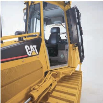
**Ease of Entry and Exit.** The hexagon shaped cab provides plenty of space to enter the roomy operator compartment. Easy to reach door handles make it easy to enter and exit during the workday. Angled doors allow the operator to walk right into the cab.
