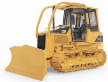
**360 Degree Guarding.** All around screen guarding is available. Canopy version includes screened, hinged doors with dampening device along with side and rear screens. The cab version offers Lexan glass doors for improved visibility while providing protection. Meets OSHA and WCB requirements.
