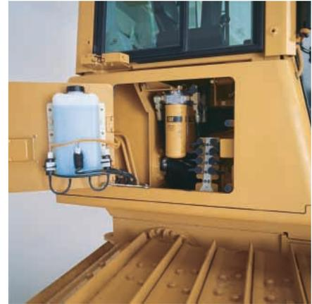
**Right Side Access Doors.** Access doors provide easy access to diagnostic test bank, hydraulic oil filters and disconnect switch.
