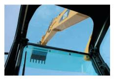
**Skylight.** A unique large polycarbonate skylight provides excellent upward visibility.
