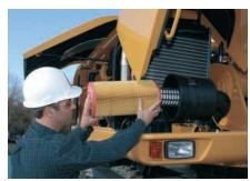
**Front Compartment.** The right front service compartment tilts providing ground level access to the batteries, ATAAC, AC condenser and the air filter.
