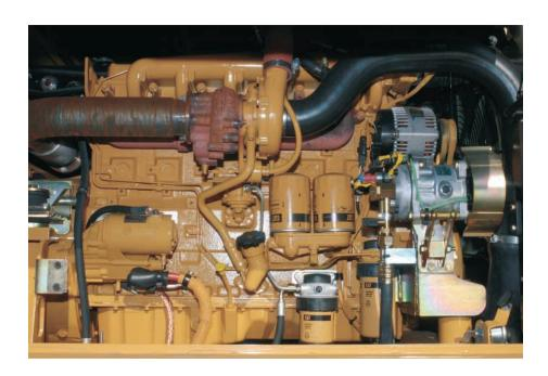
**Powerful Performance.** The 3056E DIT ATAAC engine delivers a net power of 122 kW (164 hp) at the rated speed of 2000 rpm, and meets U.S. EPA Tier 2 emission standards.
