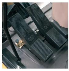
**Foot Pedals.** Two-way pedals for travel and auxiliary circuits give more floor space and reduce the need to change positions. The foot pedal for auxiliary high-pressure circuit can now be locked in the off position and is used as a footrest for greater operator comfort.
