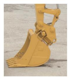
**Buckets.** Caterpillar offers four excavating buckets and four ditch cleaning buckets.
