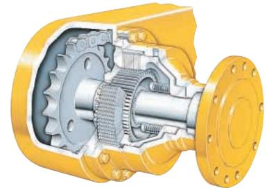
**Brakes.** Caterpillar multi-disc brakes offer a large surface area for dependable, extended-life braking. The air-actuated service brakes, located in each of the four wheel spindle housings, are sealed, adjustment free, and lubricated and cooled by tandem housing oil. The parking/emergency brakes, located in the transmission on the output shaft, are spring actuated and air pressure released. When engaged, they neutralize the transmission and lock the wheels.
