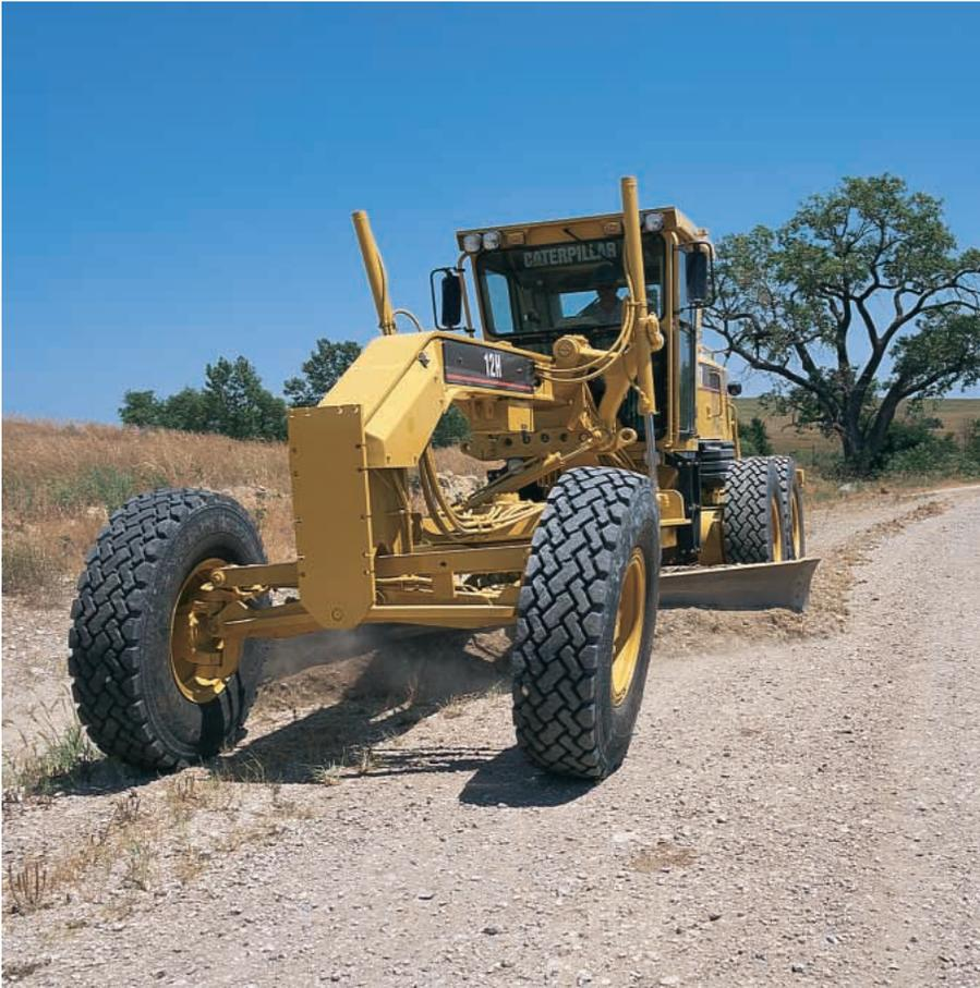
**Quiet Cab.** The resiliently mounted engine and transmission reduce interior engine noise and vibration. With the sound suppression group, interior sound levels are 75 dB(A), per ISO 6394. Lower interior noise levels improve operator working conditions.
