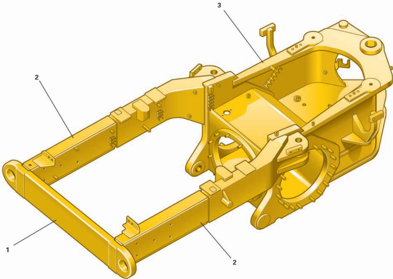
*1 Integrated bumper; 2 Box-sectioned channels; 3 Fully welded differential*
