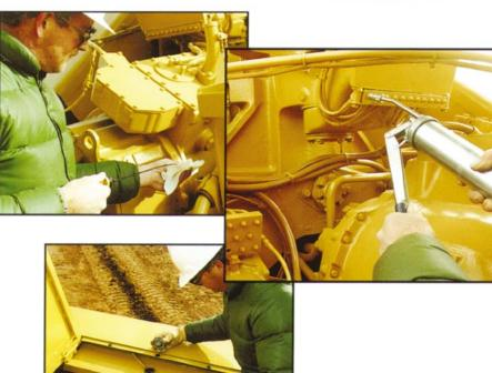
■ Maintenance platform access engine oil check and fill, engine coolant level check and fill, front brake reservoir, hydraulic system filter, secondary fuel filter.
