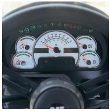
**Instrument Panel.** Redesigned instrument panel is conveniently located with easy-to-read gauges and expanded warning/indicator and diagnostic functions.
