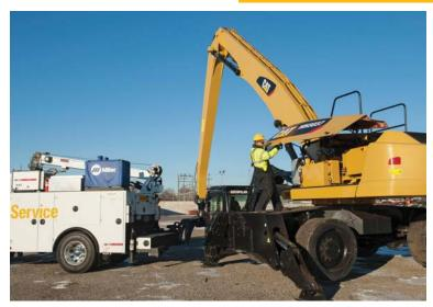
Primary service points are easily accessible through convenient access doors and platforms on the sides and top of the machine. Components can be easily located with the engine and cooling system's longitudinal layout. Access doors are hinged with supporting gas struts, ensuring that one technician can easily access all maintenance points.
