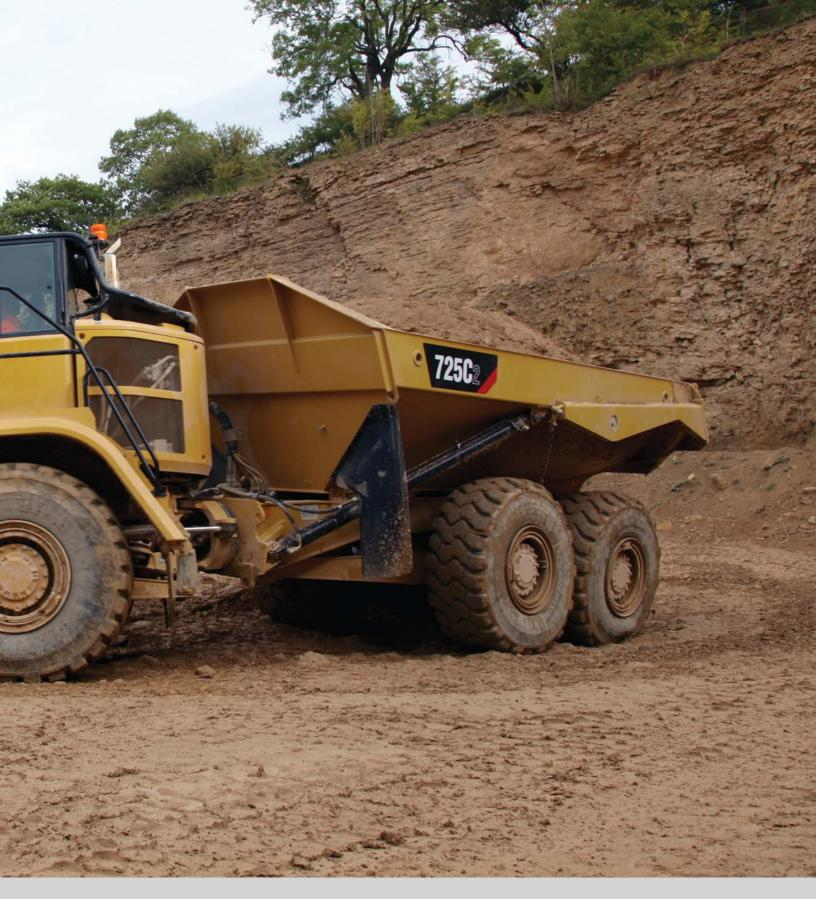
The Cat 725C2, with a 15 m<sup>3</sup> (19.6 yd<sup>3</sup>) 24 tonnes (26.5 tons) capacity, offers proven reliability, durability, high productivity, superior operator comfort and lower operating costs.
