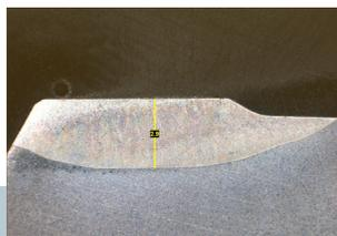
*Transverse micro-sections through the hard facing depth up to 1.0mm below the original dimension of the valve, meaning that a first regrinding step would not be possible because there is no more undercut.*
