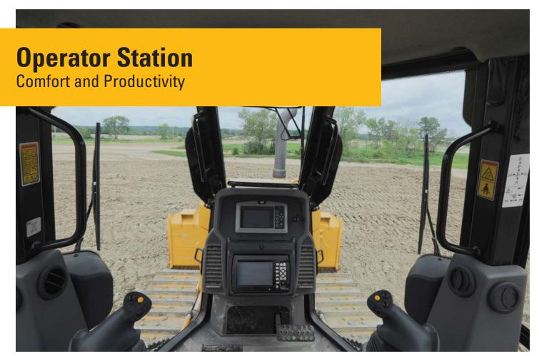
Spacious, quiet cab offers all-day comfort with wide door openings and an air suspension seat. Ergonomic, seat-mounted joystick controls isolate vibration. Excellent visibility to the blade, curbs and tight spaces help you work more precisely.
