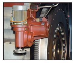
The turning device is of compact construction, safely flanged onto the engine block. An irreversible
