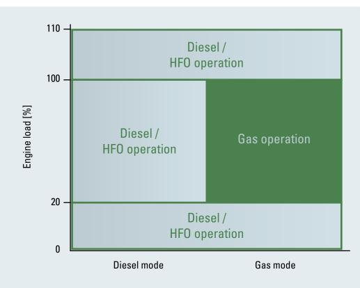
Fig. 3-5 Load restirctions in gas mode
