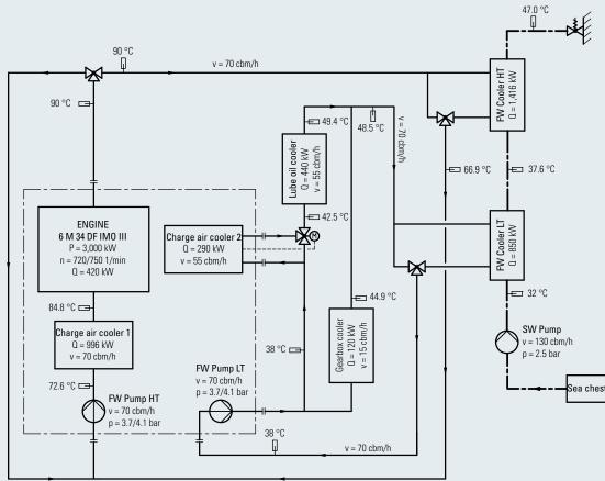
Fig. 8-9 Heat balance, system diagram 6 M 34 DF
