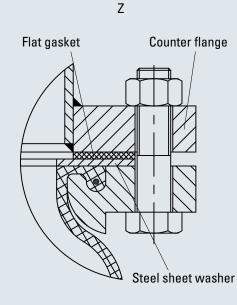
Fig. 18-2 Rubber expansion joint, detail Z
