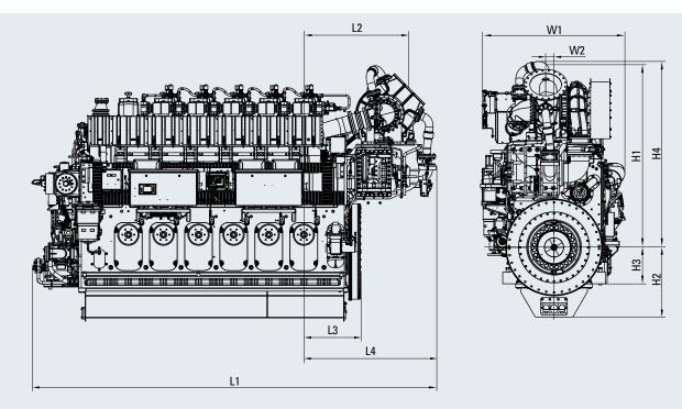
Fig. 2-2 Turbocharger at driving end – exhaust side
