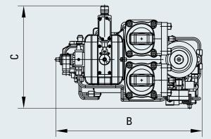
Fig. 5-18 HFO automatic filter HF4
