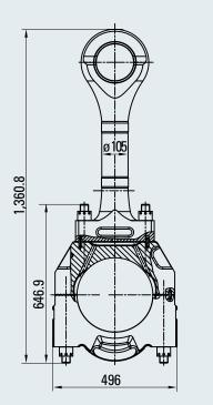
Fig. 21-6 Connecting rod, weight 224 kg
