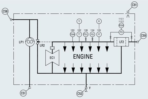
Fig. 7-1 Internal lube oil system, system diagram
