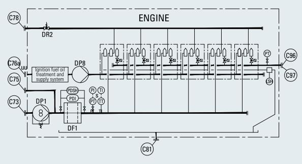
Fig. 5-1 Internal fuel oil system, system diagram
