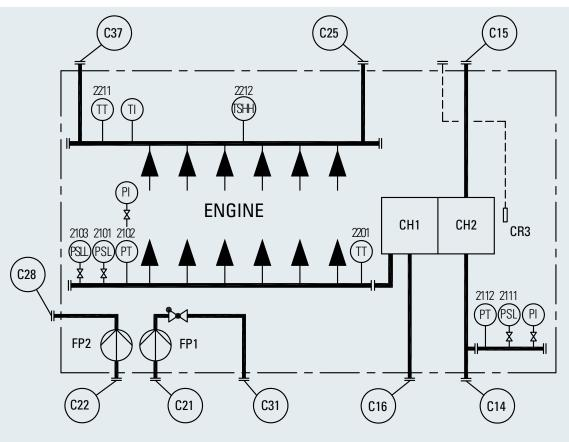
Fig. 8-1 Internal cooling water system, system diagram, turbocharger at driving end
