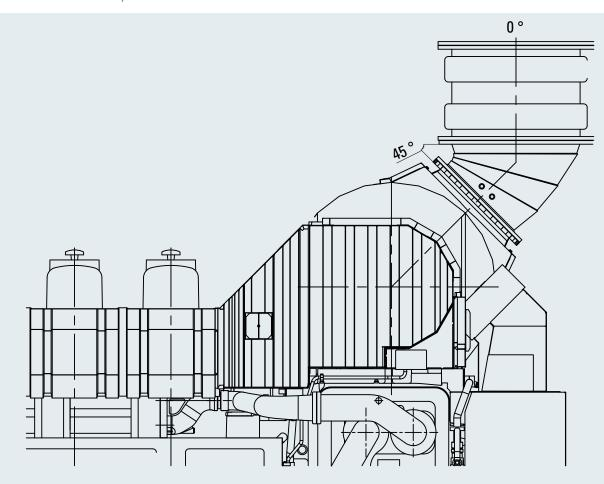
Fig. 11-3 Exhaust gas compensator
