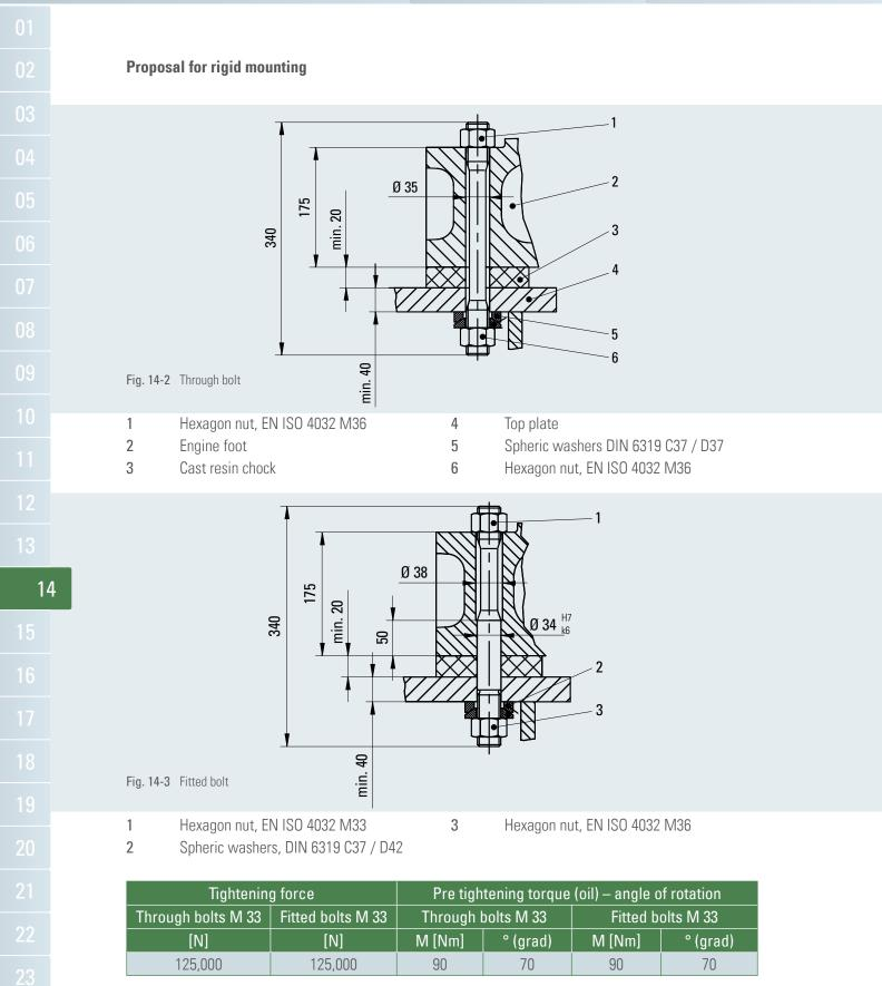
Final foundation bolts design and tightening torque by cast resin chock supplier. Design responsibility is with the shipyard.
