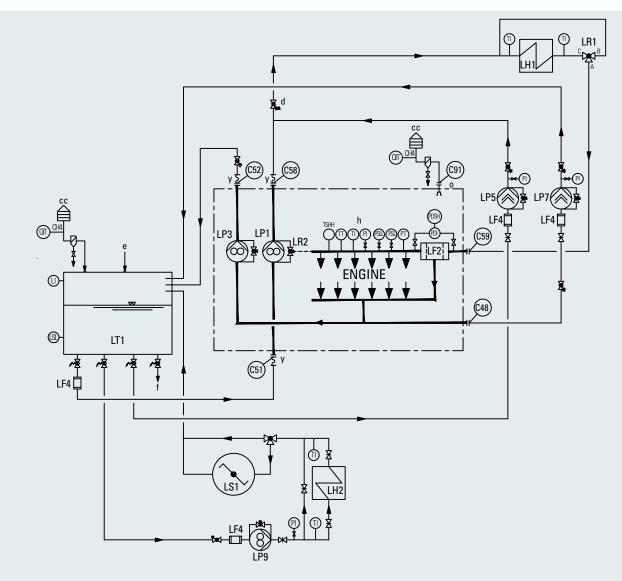
Fig. 7-12 System diagram, high level tank
