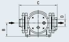
Fig. 5-20 Fuel circulating pump HP3, Stand-by circulating pump HP4
