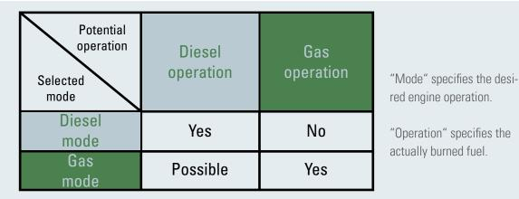
Fig. 13-8 Definition: "Mode" vs. "Operation"
