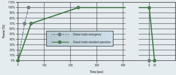
Fig. 3-2 Ramp up time M 34 DF in diesel mode
