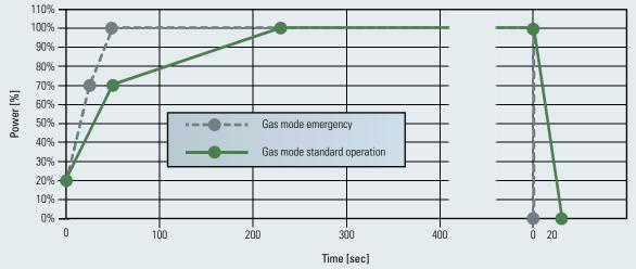
Fig. 3-3 Ramp up time M 34 DF in gas mode
