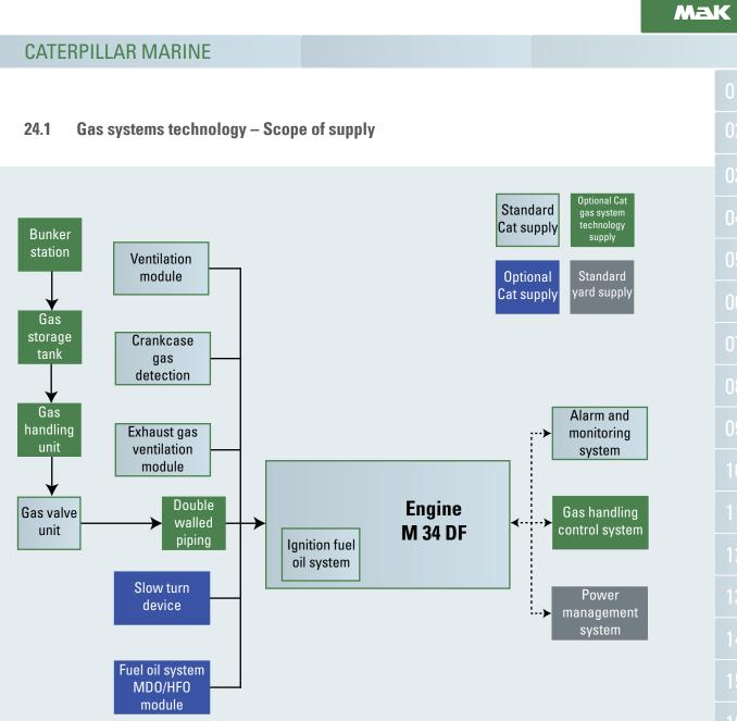
Fig. 24-1 Scope of supply M 34 DF Gas systems technology – block diagram
