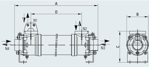
Fig. 5-8 Fuel oil cooler for MDO operation DH3
