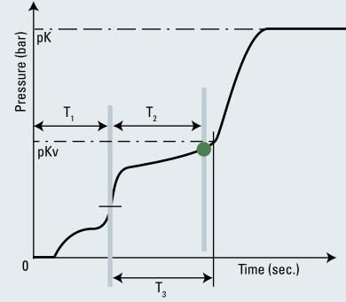
Fig. 13-7 Clutch in procedure for propulsion systems
