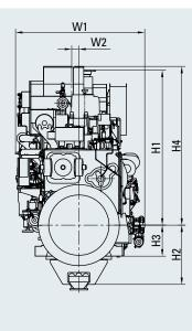
Fig. 2-1 Turbocharger at free end – control side
