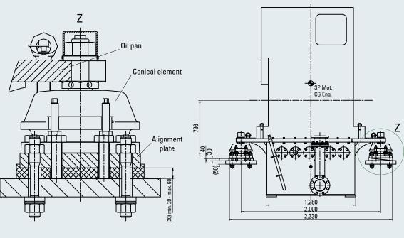
Fig. 14-6 Conical resilient element
