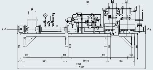
Fig. 6-4 Gas valve unit
