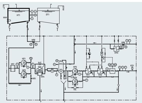
Fig. 5-23 Fuel booster and supply module, system diagram
