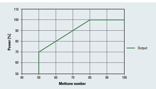
Fig. 3-7 Power as function of methane number
