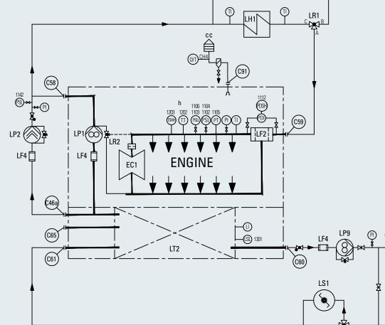
Fig. 7-11 System diagram, wet sump tank
