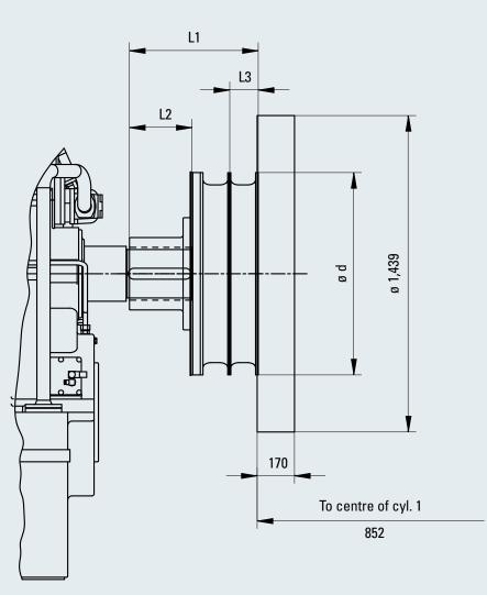
Fig. 17-1 Flywheel and flexible coupling
