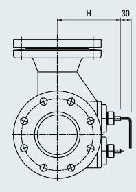
Fig. 7-9 Lube oil temperature control valve LR1
