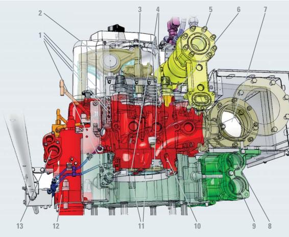
Fig. 1-4 Cylinder head
