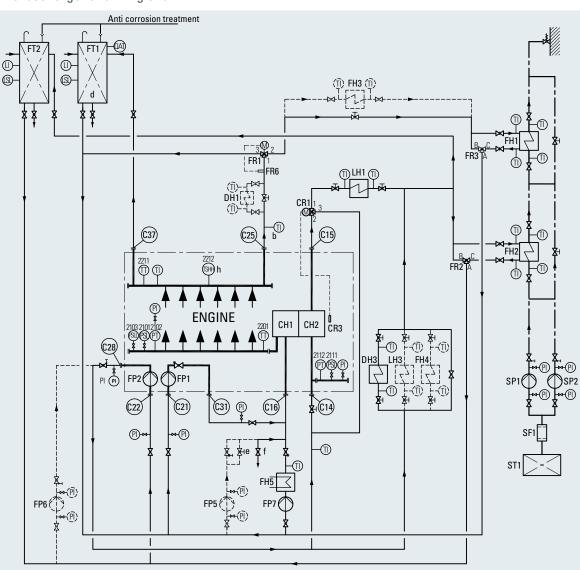
Fig. 8-3 External cooling water system, system diagram, turbocharger at driving end
