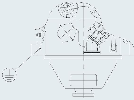
Fig. 14-7 Earthing connection on the engine
