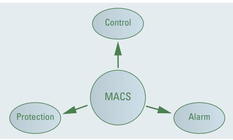
The M 34 DF engines will be provided with a new Modular Alarm and Control System, called MACS. The basic engine control and monitoring system will be installed in the local control panel. Where extension modules are necessary external plc based I/O extension modules will be installed.
