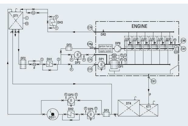
Fig. 5-3 External fuel oil system diagram without intermediate tank
