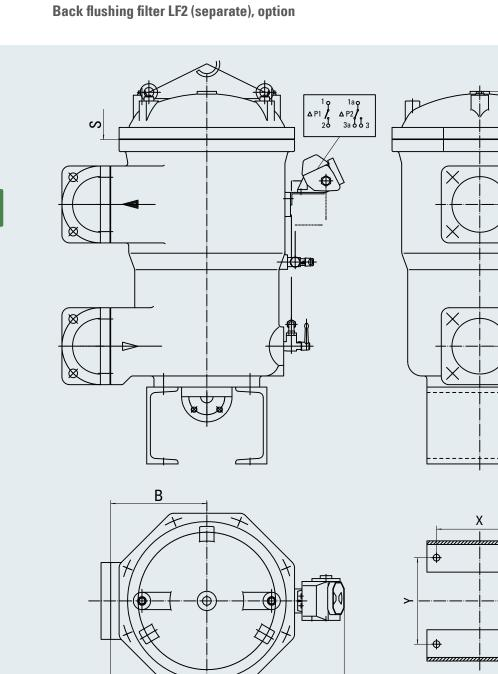
Fig. 7-3 Back flushing filter LF2
