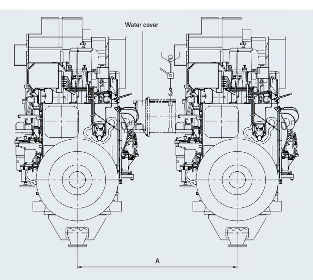
Fig. 19-1 Center distance of twin-engine plants
