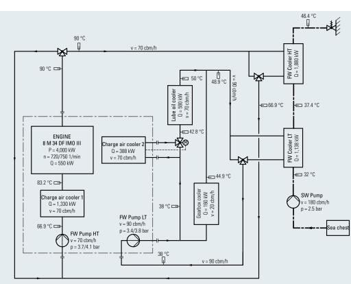
Fig. 8-10 Heat balance, system diagram 8 M 34 DF
