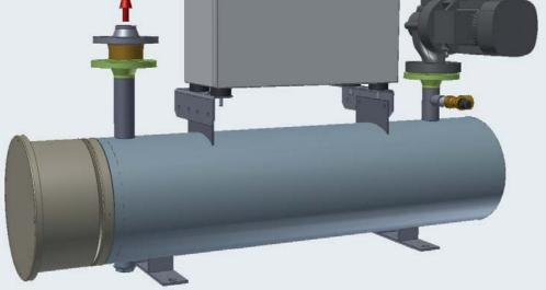
Fig. 8-12 Freshwater preheater FH5, preheating pump FP7
