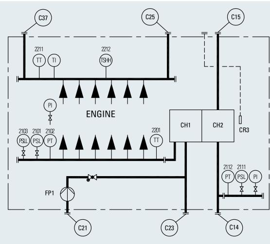
Fig. 8-2 Internal cooling water system, system diagram, turbocharger at free end
