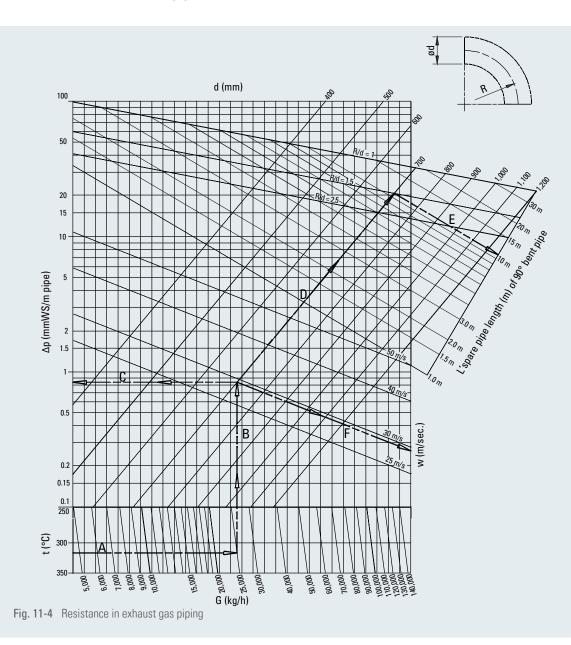
Example (based on diagram data A to E): T = 335 °C, G = 25,000 kg/h L = 15 m straight pipe length, d = 700 mm 3 off 90 ° bend R/d = 1.5 1 off 45 ° bend R/d = 1.5  $\Delta$ Pg = ?
