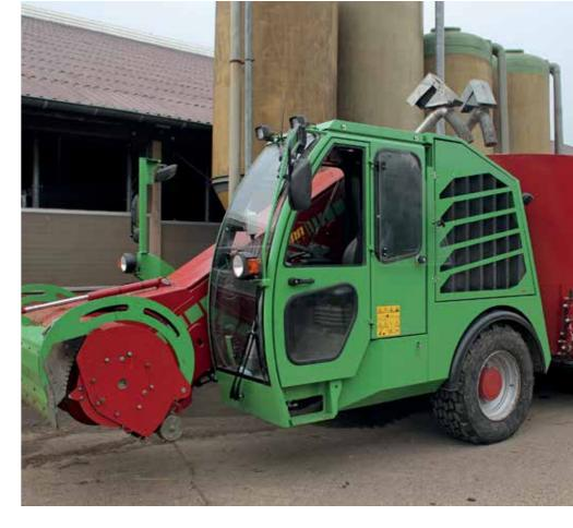
equipped with a standard rigid front axle with front-wheel drive and a controlled swing axle at the rear. It is
