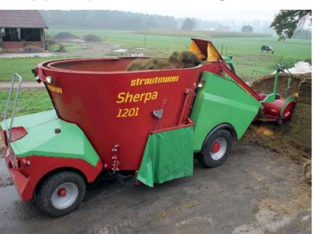
driven by a 4 cylinder 1104D-44TA Perkins engine, delivering 106 kW (144 hp) at 2200 rpm, and the standard maximum speed is 15 km/h. A 25 km/h registration tin combination with a hydraulic chassis suspension is available as an optional extra. The self-propelled Sherpa model discharges the mixed fodder via side doors with adjustable discharge chutes or optional PVC discharge conveyors.
