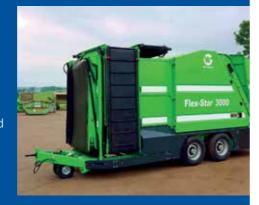
The Flex-Star 3000 is built on an 80 km/h-chassis with a serial compressed air system and ABS, so it's quick to transport to where
