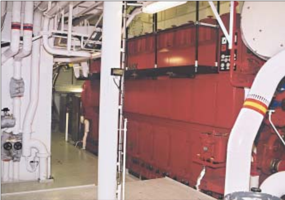
The propulsion plant consists of two MaK 9M32 medium-speed non-reversible diesel engines
