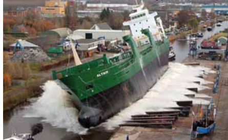
'Altair' was launched sideways into a very narrow canal in the standard Bodewes Shipyards fashion
