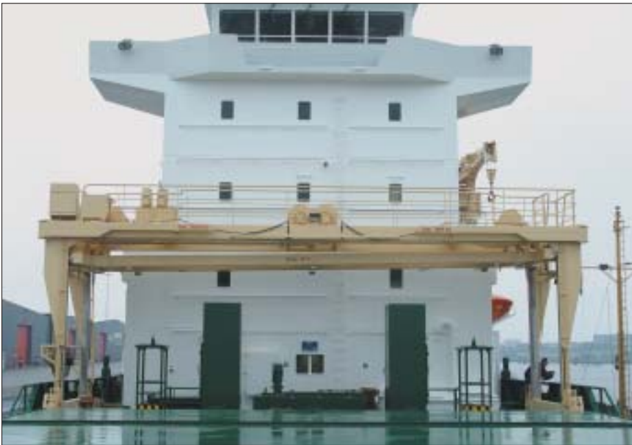
The hatches are handled by a Coops & Nieborg gantry crane
