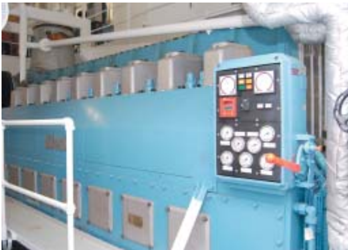
The MaK main engine puts out 2970 kW
