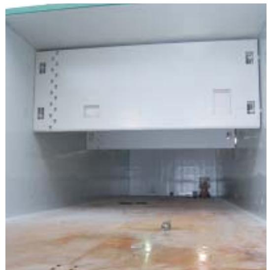
The hold can be divided with grain bulkheads
