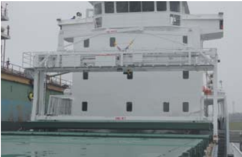
The gantry crane just picked up a hatch cover
