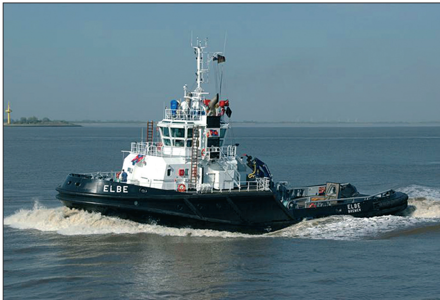
Elbe , one of a pair of Voith Schneider tugs for German ports built by Zamakona.
