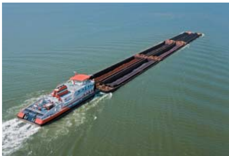
The 'Veerhaven X - Orka' pushing 6 loaded barges at 18.5 km/h
