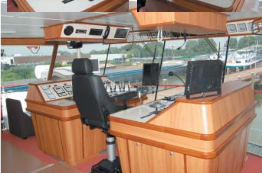
To improve the view forward, the bridge windows are without mullions
