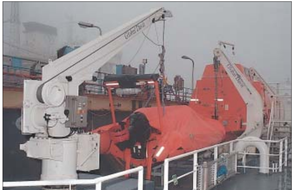
The lifeboats are launched and recovered with deck-mounted hydraulically operated folding davits
