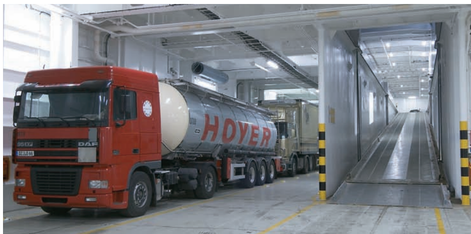
Roro access equipment has been delivered by MacGregor and includes one internal hoistable ramp leading from deck 3 to deck
