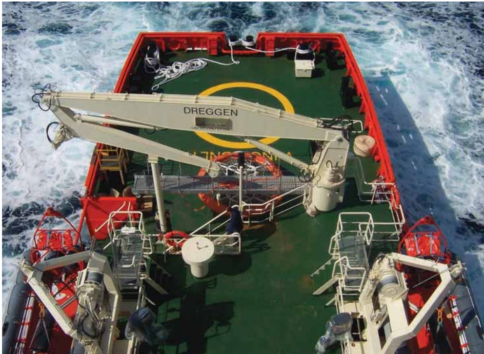
The crane is used to deploy rescue scoops during rescues
