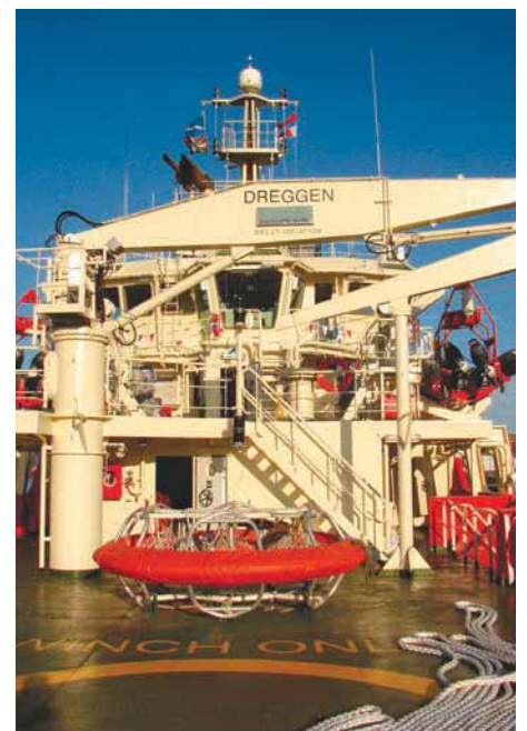
Rescue equipment includes two FRCs, a Dacon scoop and a Cosalt rescue basket
