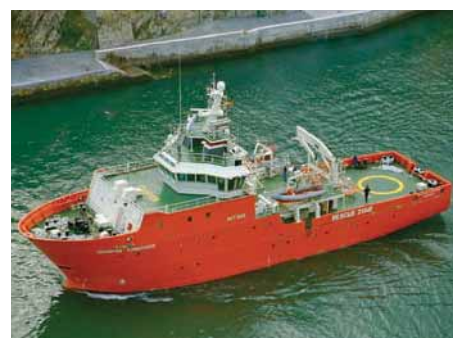
The deckhouse front on the forecastle deck shields the wheelhouse from green water
