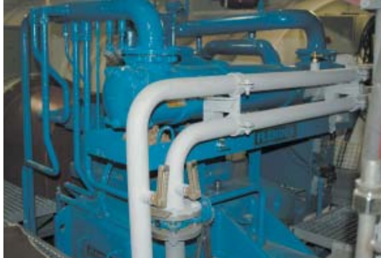
The Flender reduction gearbox with secondary PTO
