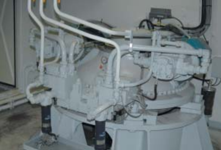
The steering is handled by a electro-hydraulic steering gear
