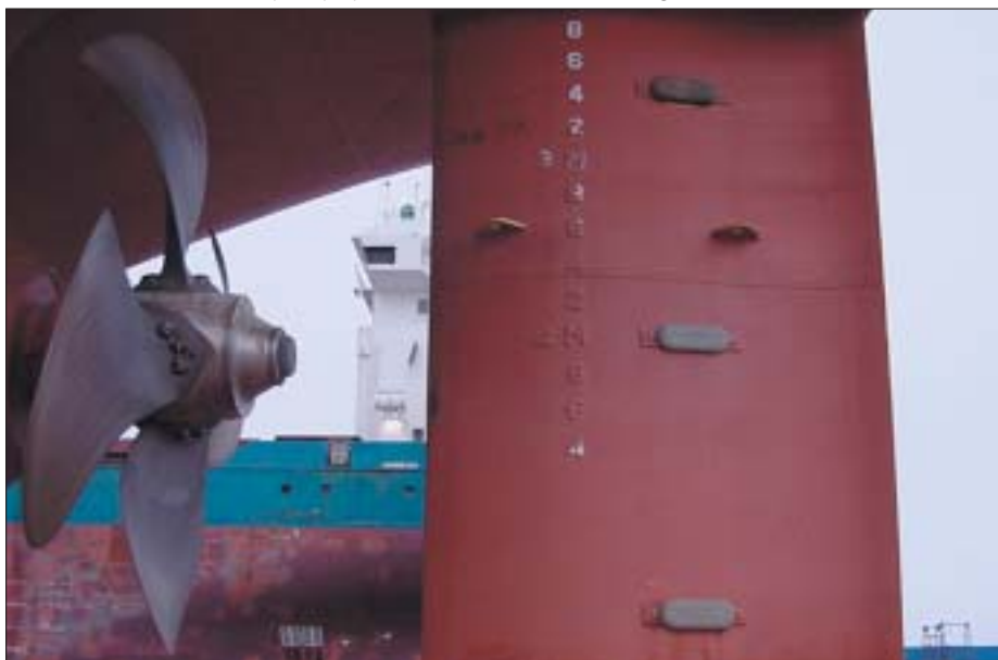
The Scana Volda controllable pitch propeller and the Van der Giessen large size rudder
