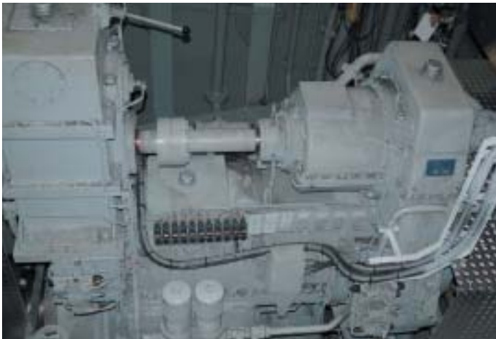
The Scana Volda reduction gearbox featuring pto/pti
