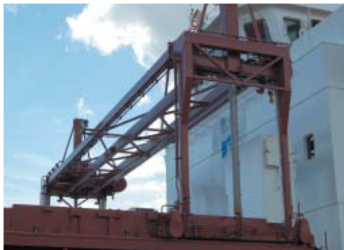
The hatch covers are handled with a gantry crane
