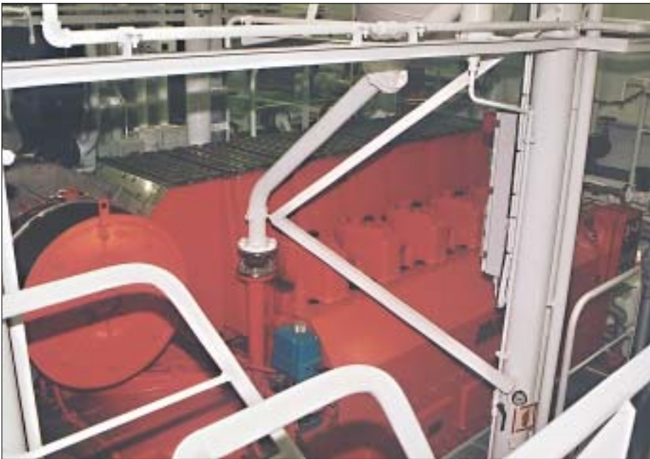
The propulsion plant consists of a MaK marine diesel engine, type 6M25
