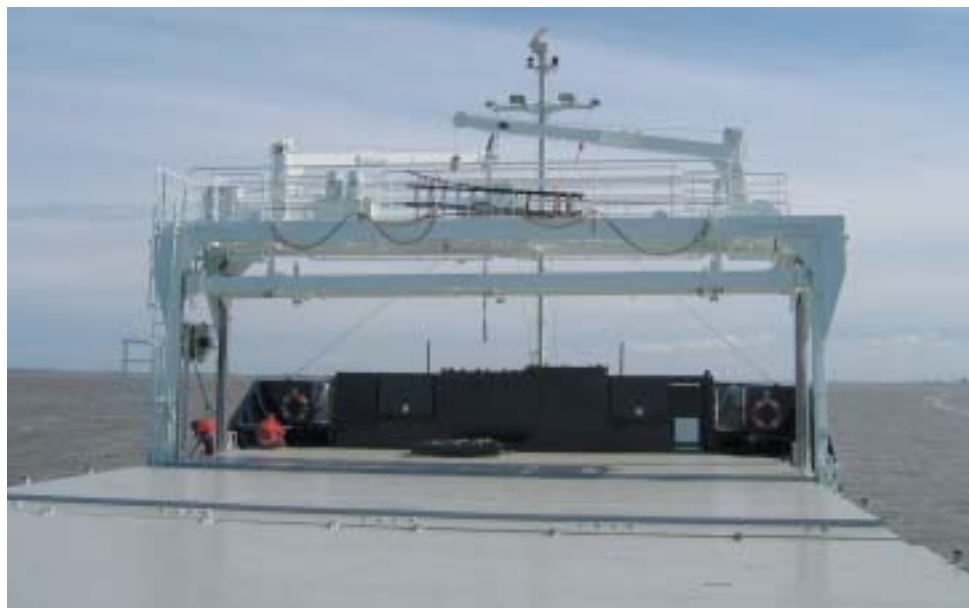
The hatch covers are manoeuvred by a travelling gantry crane
