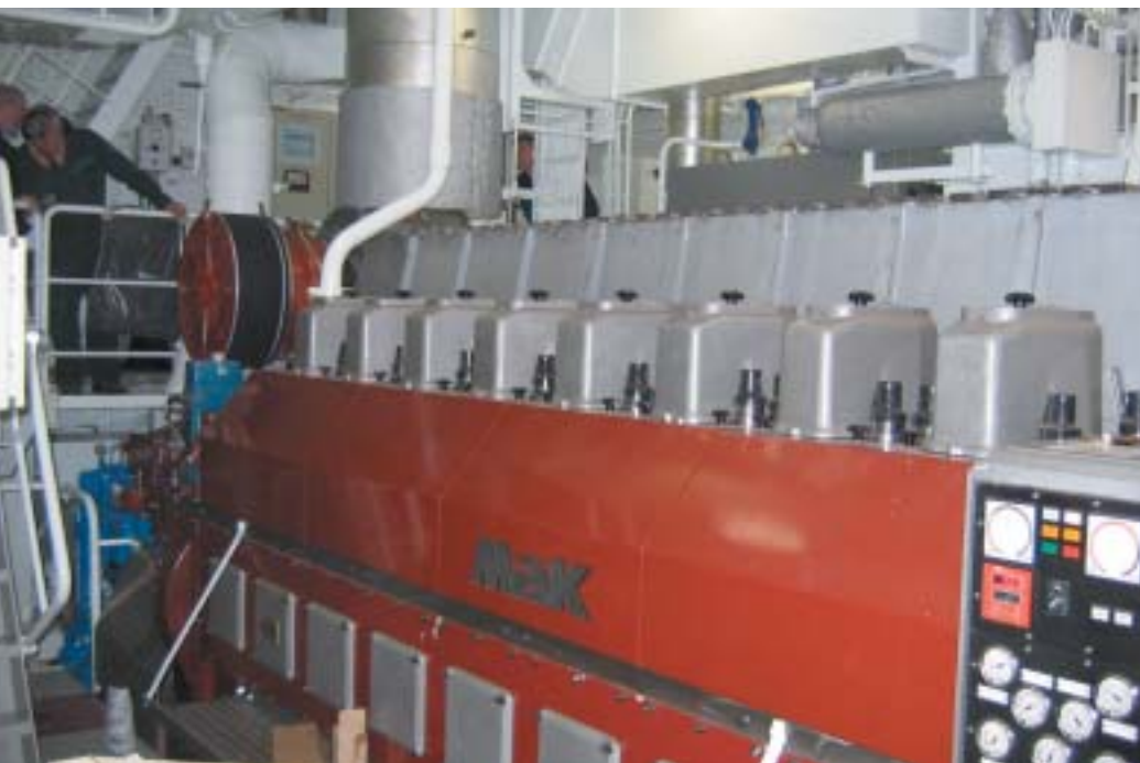
A MaK diesel engine delivers 2640 kW of propulsion power
