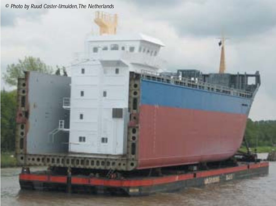
The superstructure was transported inside one of the hull sections
