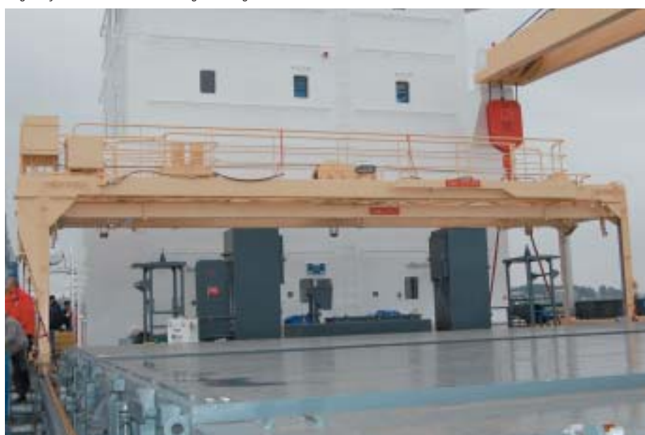
A gantry crane is used for moving the cargo hatches and the tweendeck
